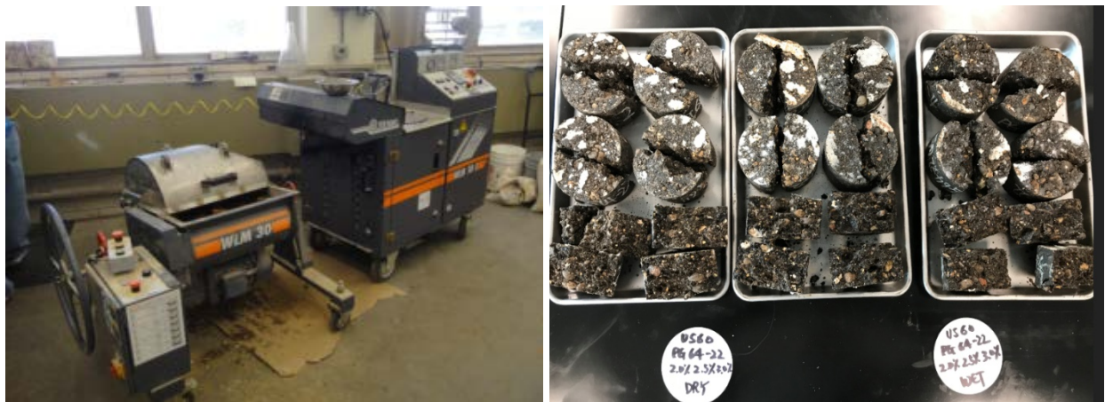
Figure 26. Lab Foaming Equipment and CIR Specimens after IDT Test.
