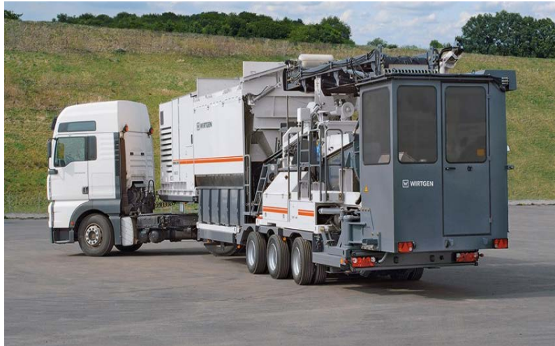
(a) Wirtgen: mobile cold recycling mixing plant
