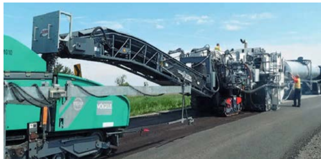
(a) Wirtgen 2200 CR: track-mounted recycler
