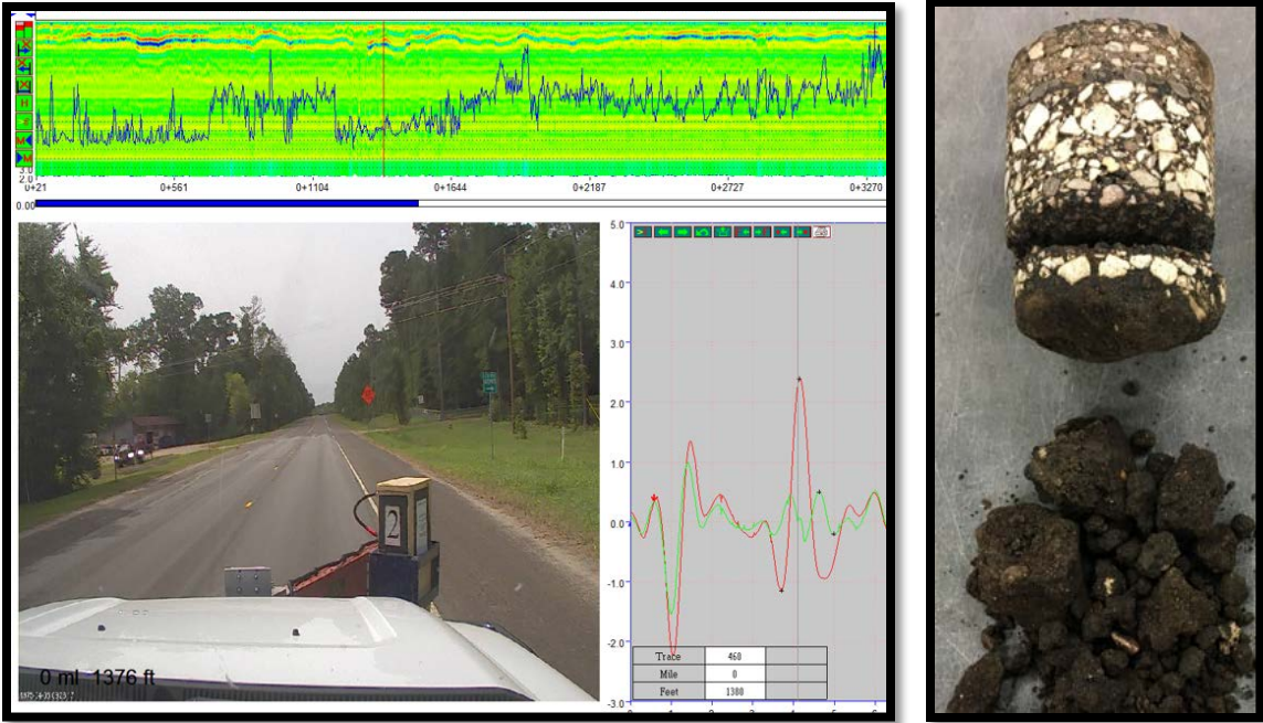
Figure 24. Example GPR and Core from FM 92.
