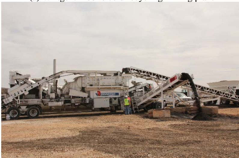
(b) Roadtec: mobile cold recycling mixing plant
