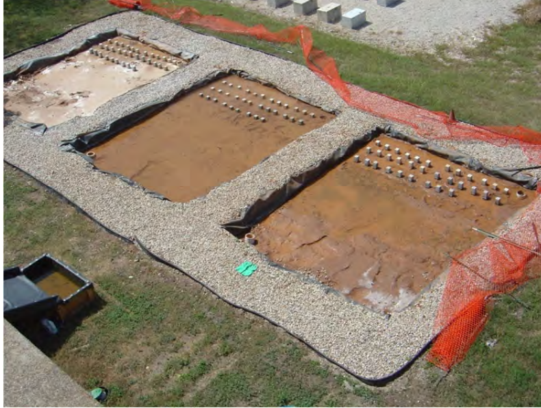
Figure 5.1: Outdoor sulfate exposure site located in Austin, TX. From left to right, the trenches contain calcium sulfate, sodium sulfate, and magnesium sulfate.
