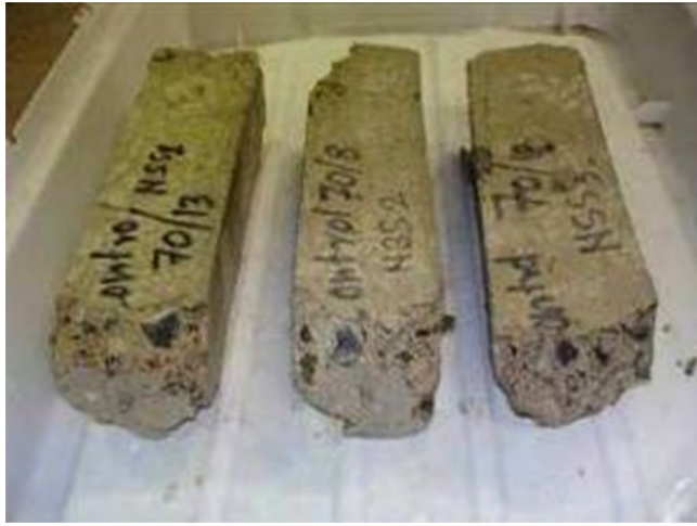
w/cm = 0.70, 200 days in \text{Na}_2\text{SO}_4
