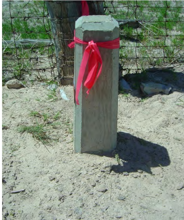
Figure 7.16: New ROW marker with Class C fly ash at 0.4 w/cm after 3 months of exposure in gypsiferous soils
