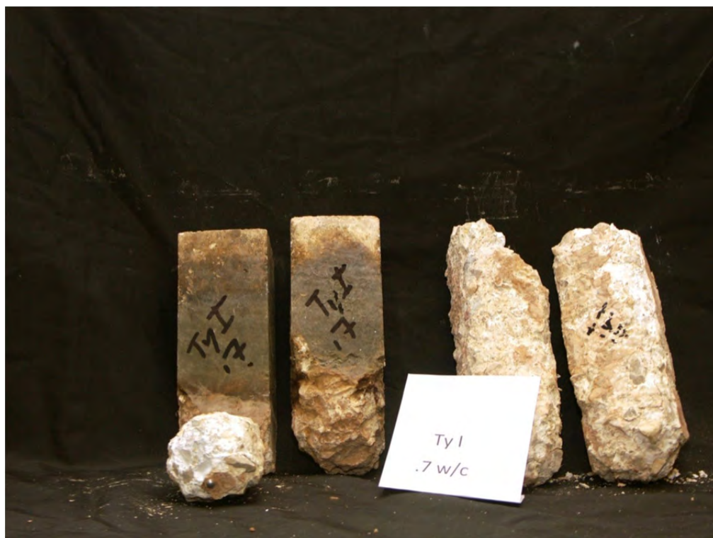
Figure 5.13: Concrete Prisms Exposed to 33000 ppm Calcium Sulfate, Type I Cement at 0.7 w/cm
