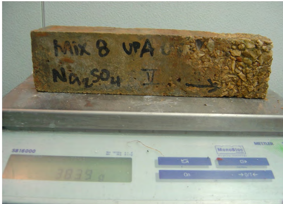
Figure 5.16: Mixture C5-7 after 18 months of outdoor exposure to sodium sulfate. This prism was placed vertically, with the section on the left fully submerged below sulfate-saturated soil.
