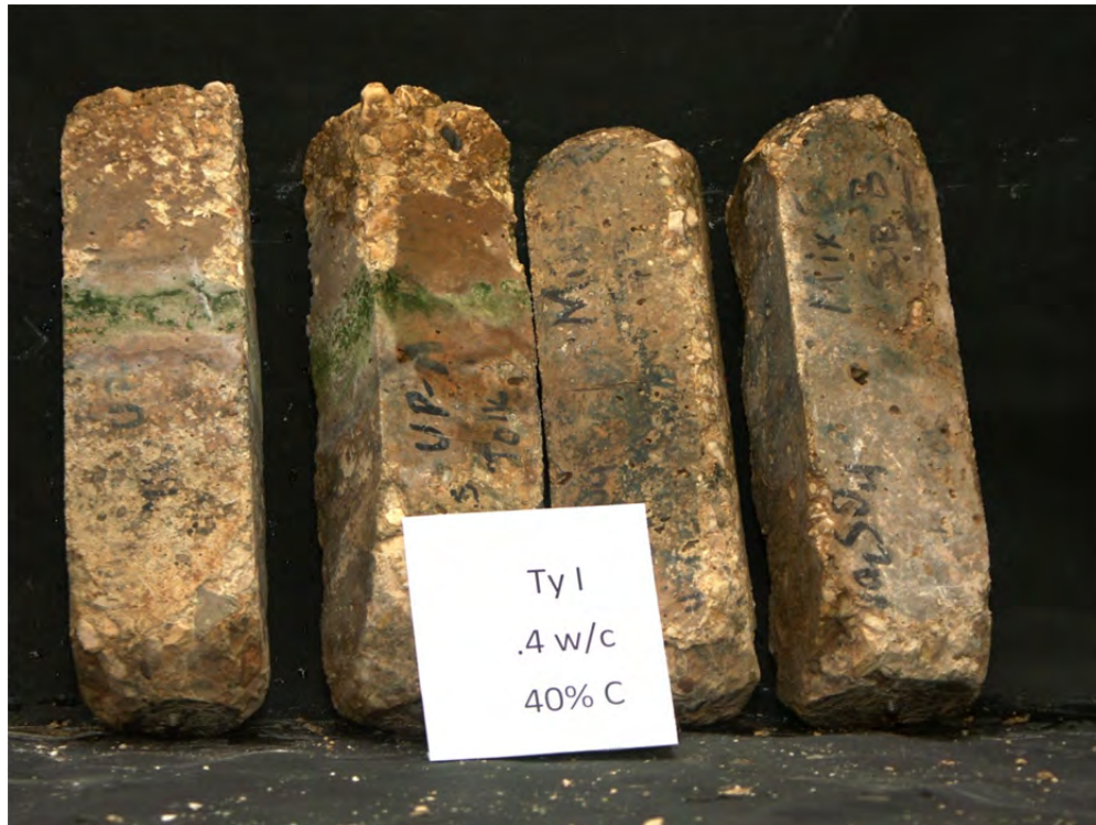
Figure 5.22: Damage to prisms exposed to 33000 ppm sodium sulfate
