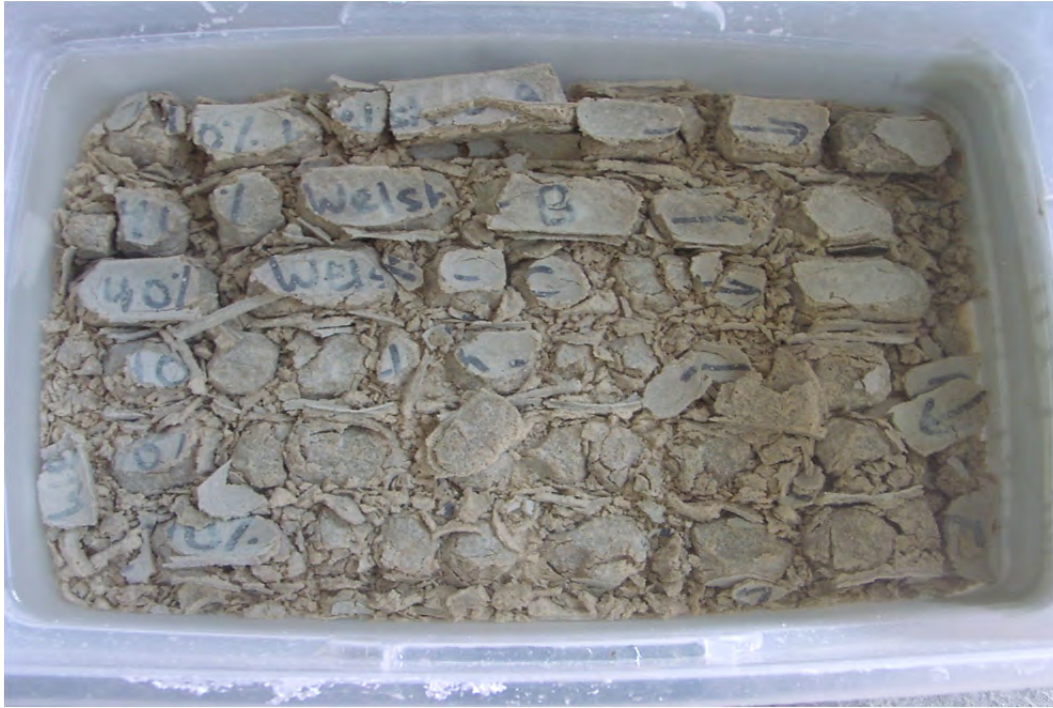
Figure 4.6: FA8 after 56 days in ASTM C 1012 testing
