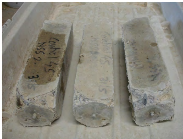
w/cm = 0.45, 280 days in \text{Na}_2\text{SO}_4
