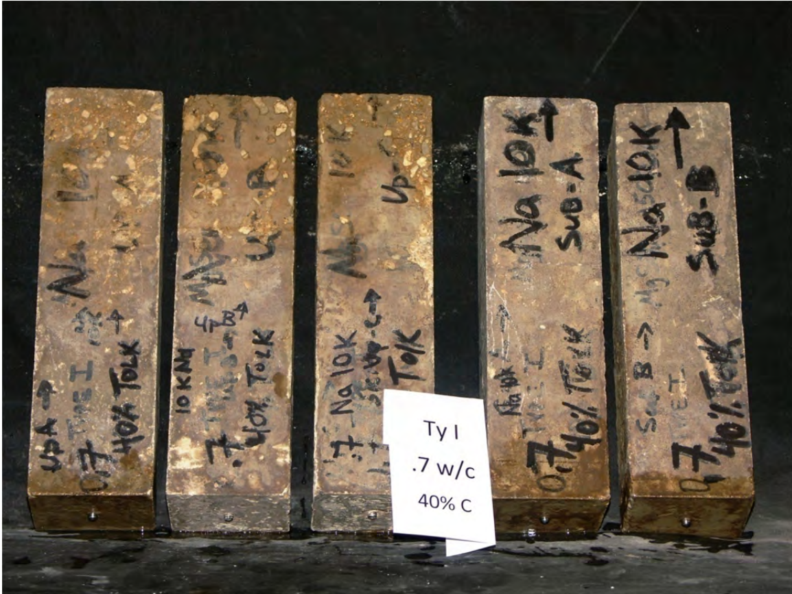
Figure 5.33: Physical Sulfate Attack in 10000 ppm Sodium Sulfate Above Soil Contact Zone
