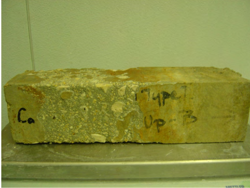
Figure 5.7: Concrete prism with a 0.4 w/cm placed vertically in the outdoor calcium sulfate exposure site. In this photograph, the left side shows the portion of the prism that was below the soil level.
