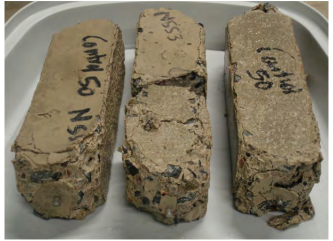
w/cm = 0.50, 320 days in \text{Na}_2\text{SO}_4
