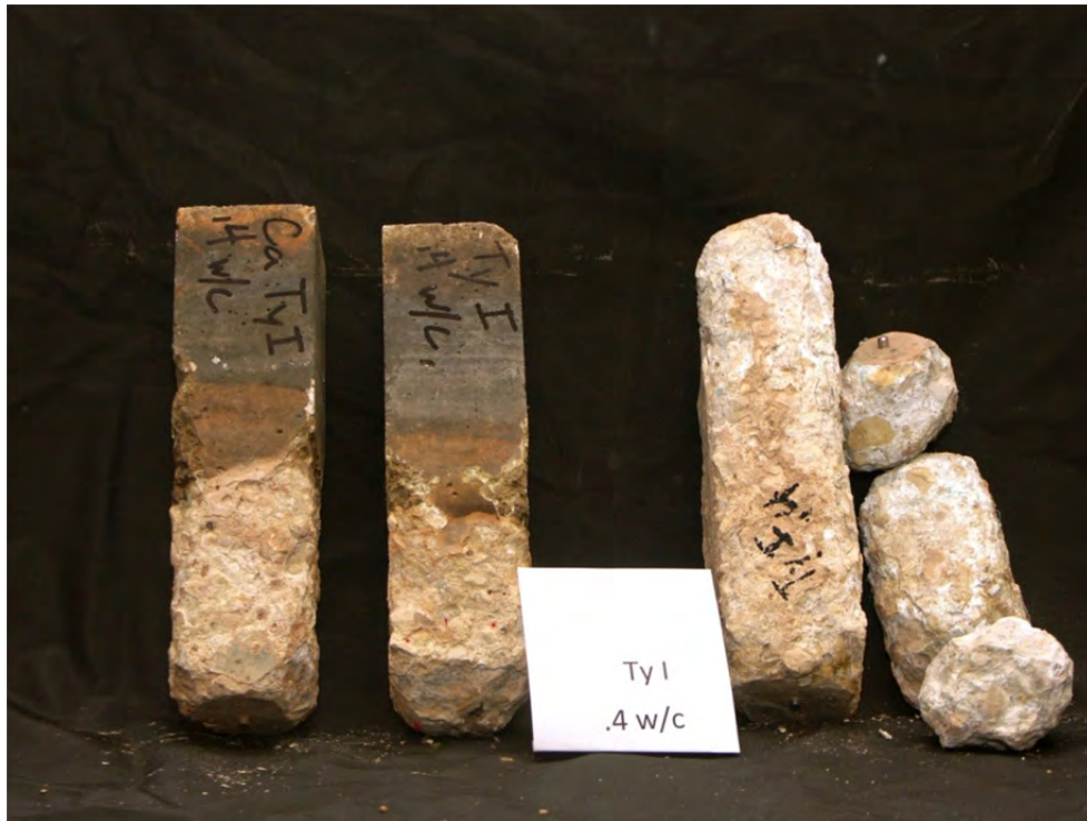
Figure 5.12: Concrete Prisms Exposed to 33000 ppm Calcium Sulfate, Type I Cement at 0.4 w/cm
