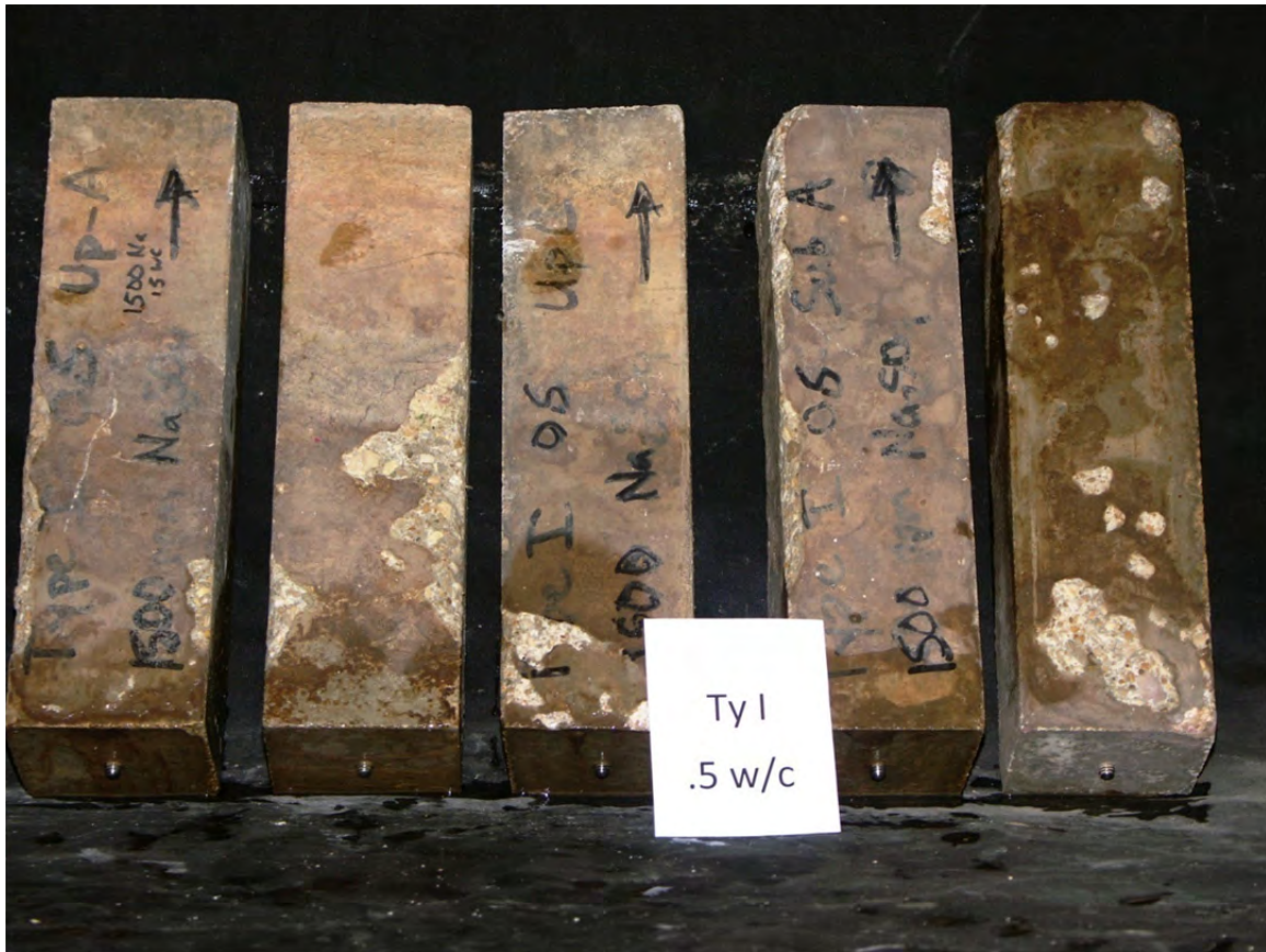
Figure 5.31: Surface Scaling in 1500 ppm Sodium Sulfate in Soil Contact Zone
