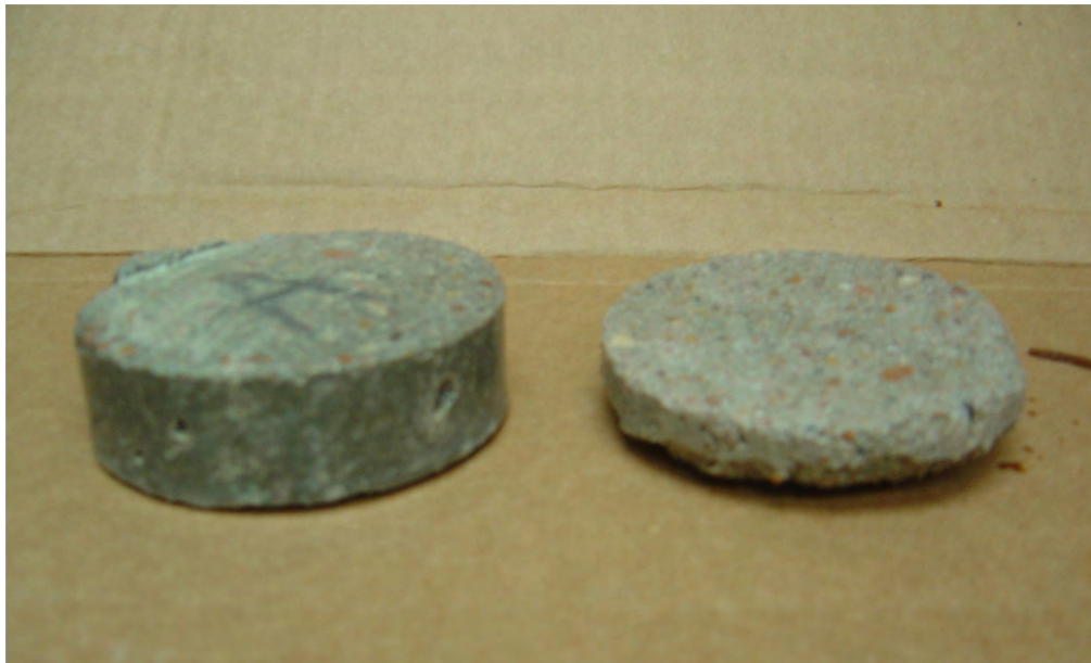
Figure 5.36: Mortar specimens before and after physical sulfate testing. The mixture contained Type V cement at 0.7 w/cm . The disk on the left was prior to testing and the disk on the right went through 150 cycles.
