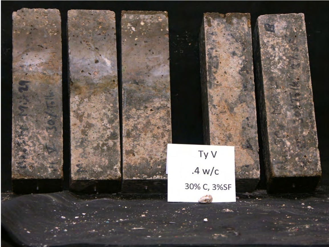
Figure 5.24: Concrete Prisms Exposed to 33000 ppm Sodium Sulfate exhibiting excellent performance
