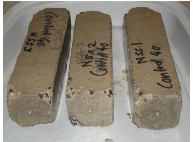
w/cm = 0.40, 520 days in \text{Na}_2\text{SO}_4
