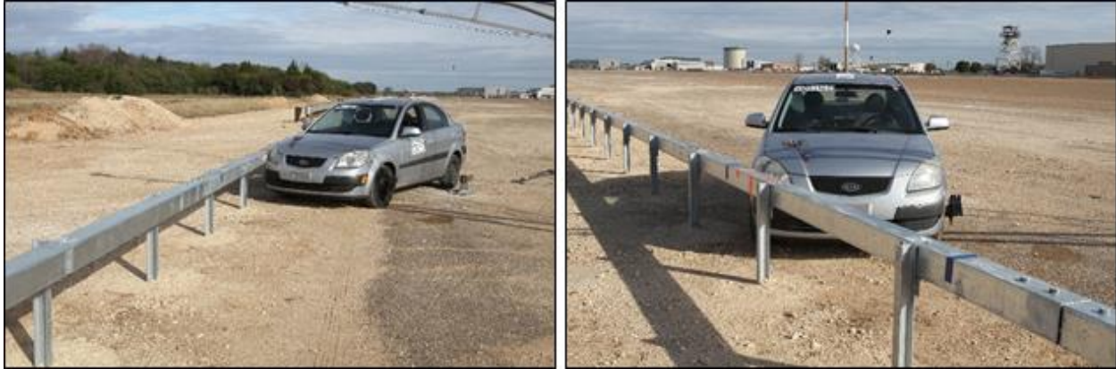
Figure 5.1. Barrier/Test Vehicle Geometrics for Test No. 610031-01-1.
