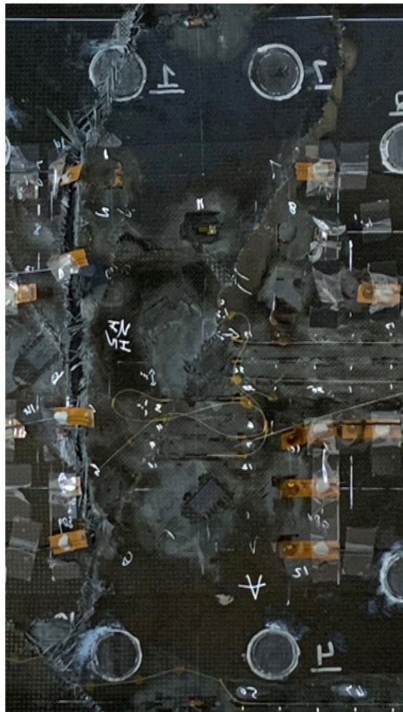
Figure E 11. Post-failure images of panel 5
