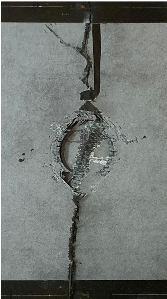
Figure E 11. Post-failure images of panel 5
