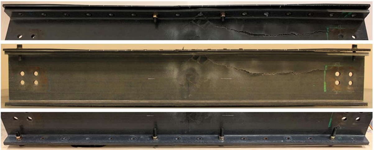
Figure E 3. Post-failure images of panel 3 and side-channels
