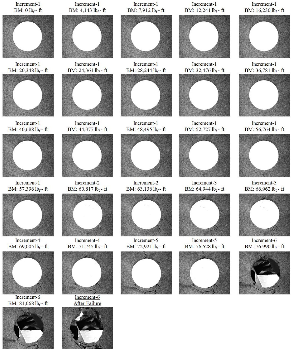
Figure E 13. Panel 4 visual results using NFOV camera during residual strength test
