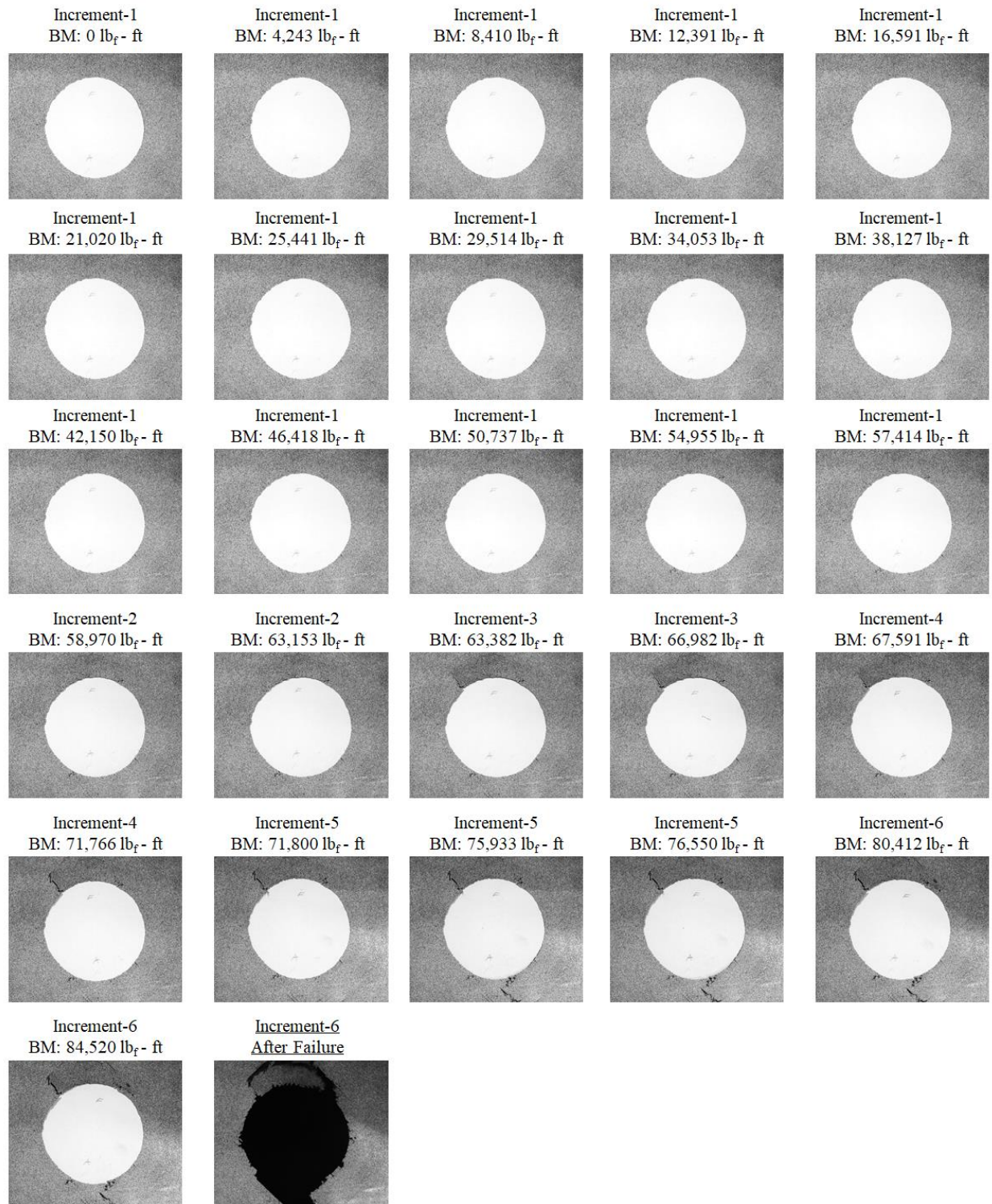
Figure E 18. Panel 6 visual results using NFOV camera during post-fatigue residual strength test
