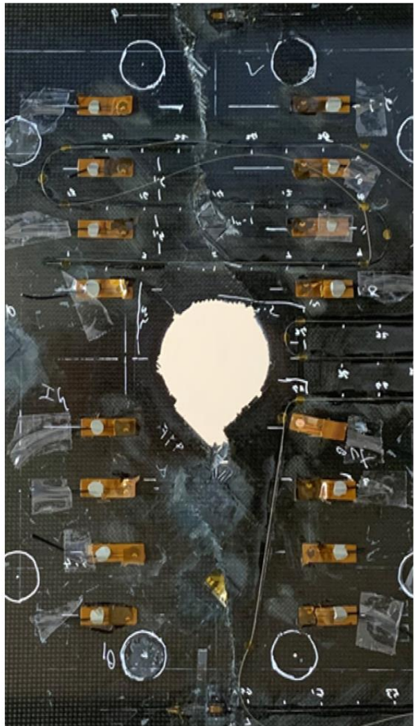
Figure E 20. Post-failure images of panel 6
