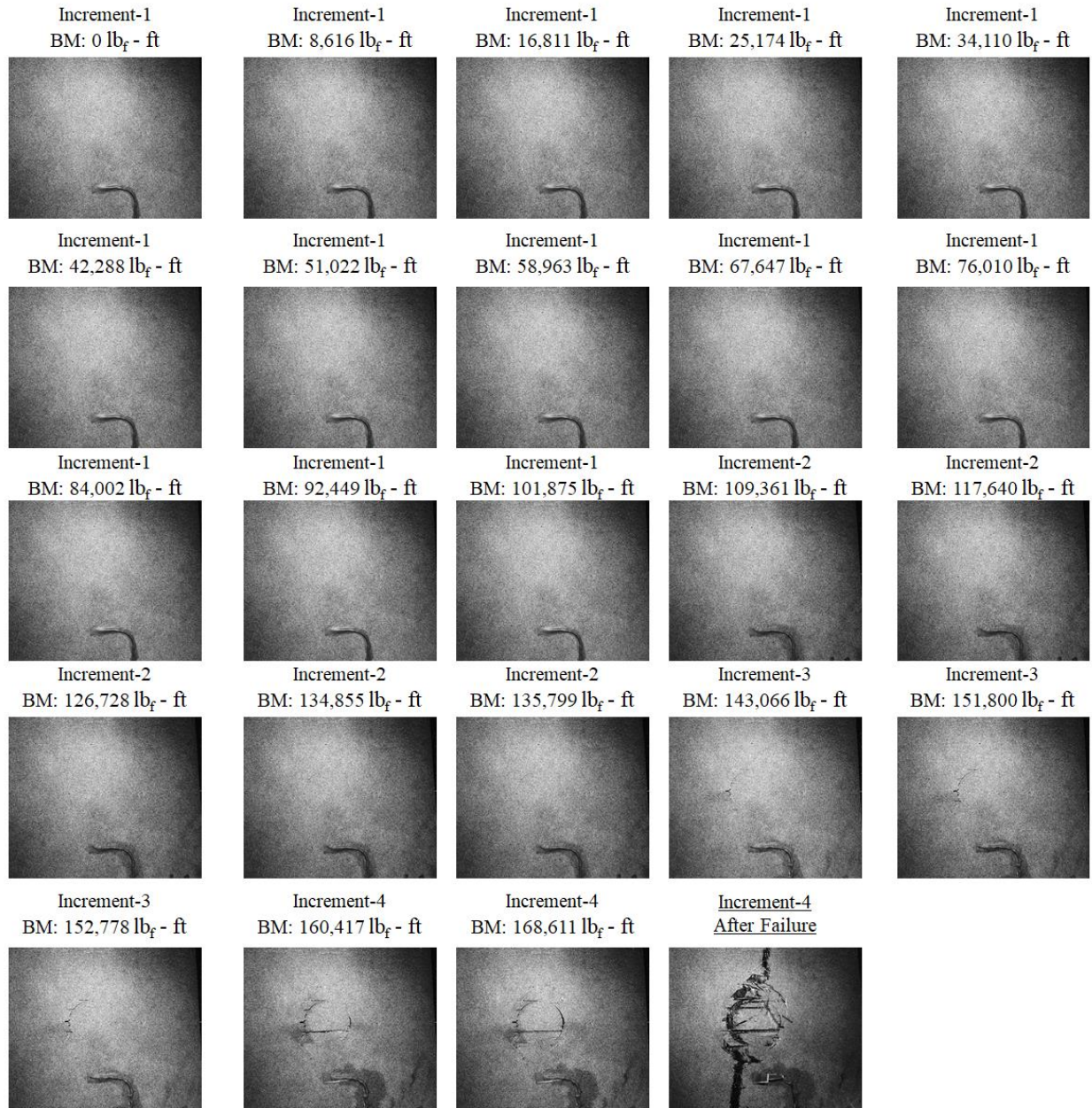
Figure E 1. Panel 3 visual results using WFOV camera during residual strength test
