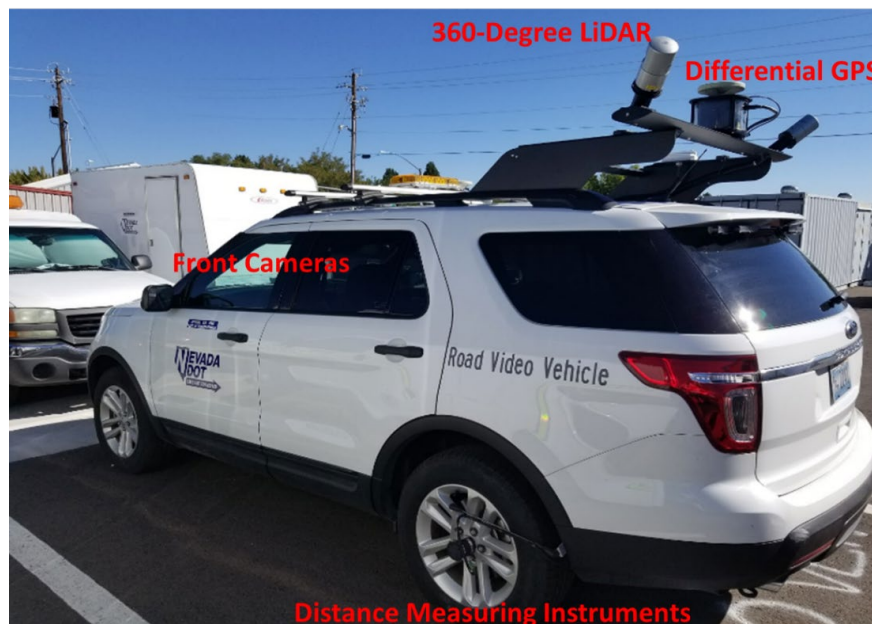
Figure 1. NDOT road video vehicle equipped with differential sensors.
