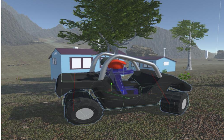
Figure 3-3: Glowing lines show how each wheel is modelled as a spherical collider on a suspension.
