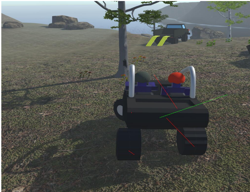
Figure 3-4: Current force on each wheel is shown in red, and net force on the vehicle in green
