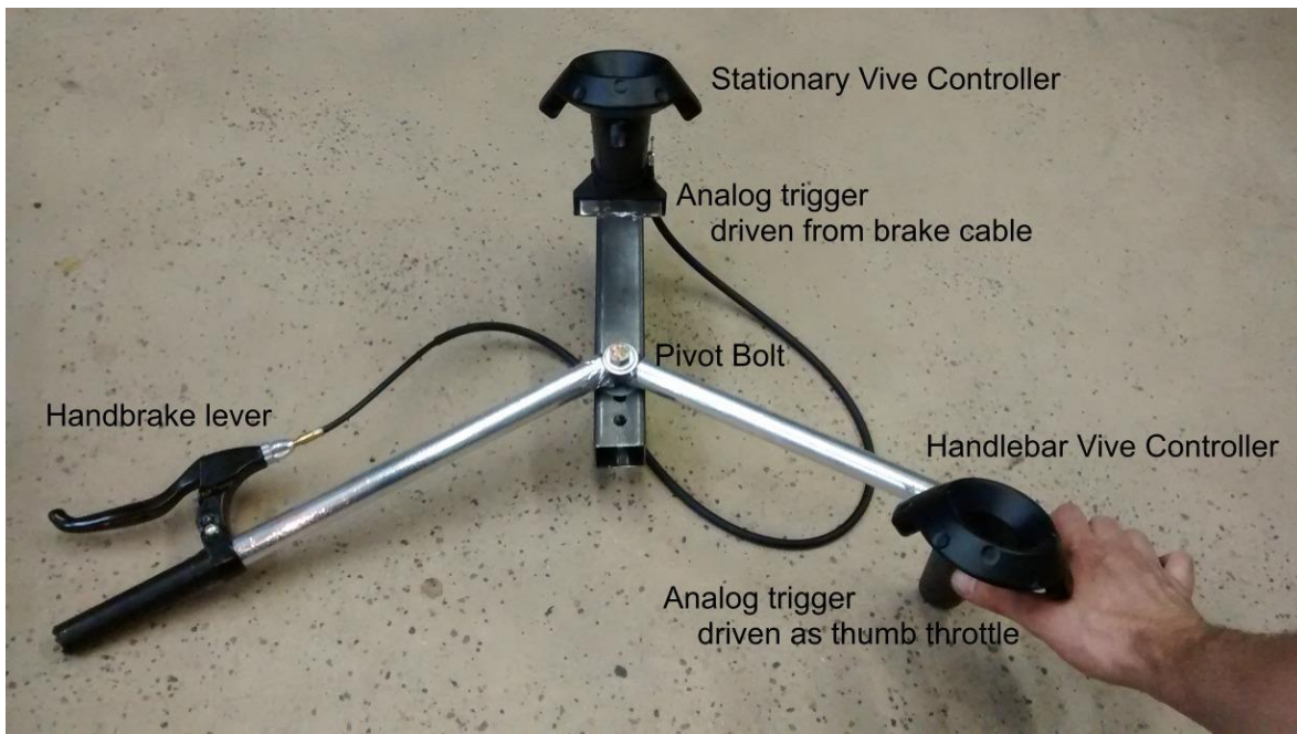
Figure 3-2: An early prototype of a VR input device modeled after ATV handlebars
