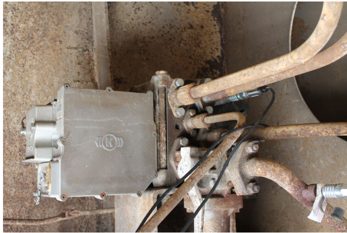
Figure 16 – Vendor CCD Installed on Test Car #2 (IN 941)
