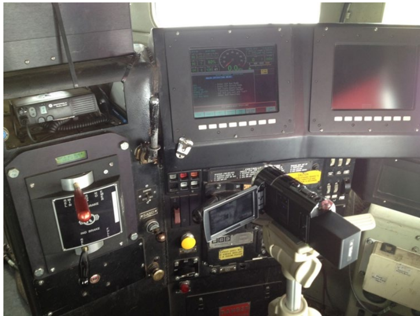
Figure 8 – Vendor’s ECP Brake with Integrated HEU in DOTX-2000
