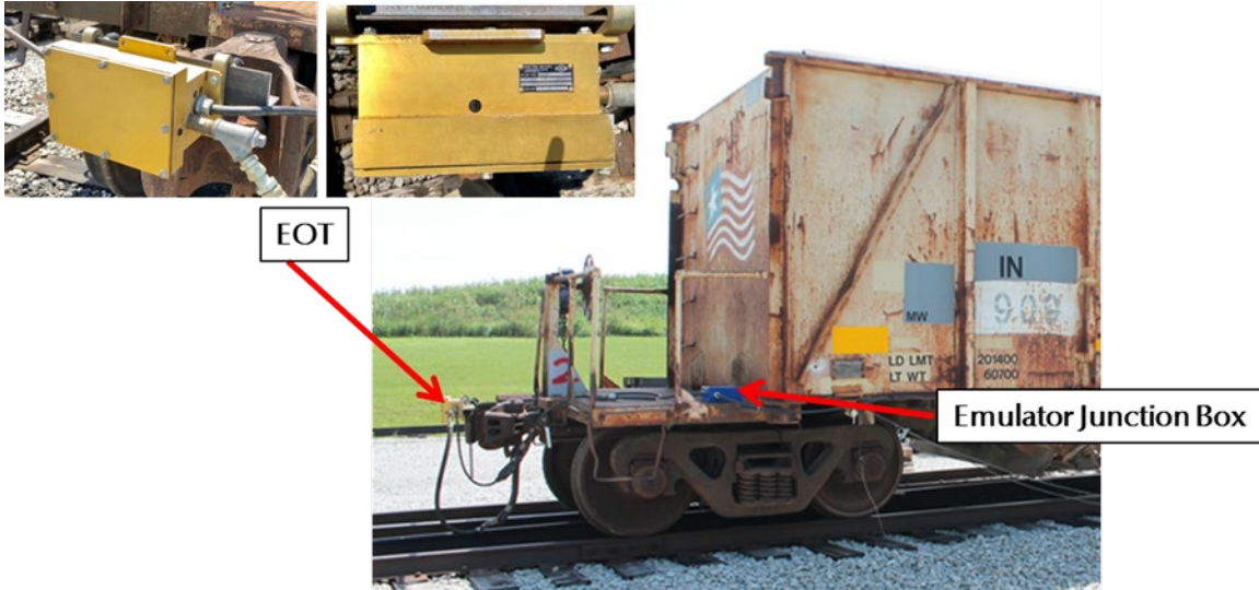
Figure 18 – Vendor ECP EOT and Emulator Junction Box on Test Car #3 (IN 909)
