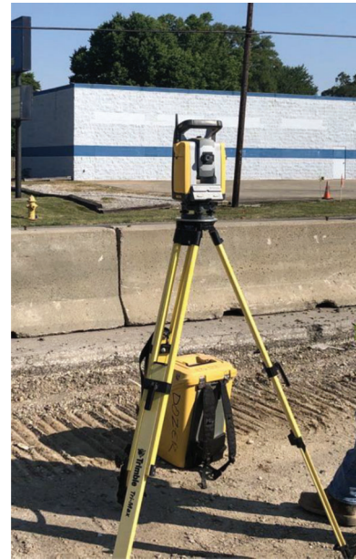
Figure 4.14 Robotic total station.
