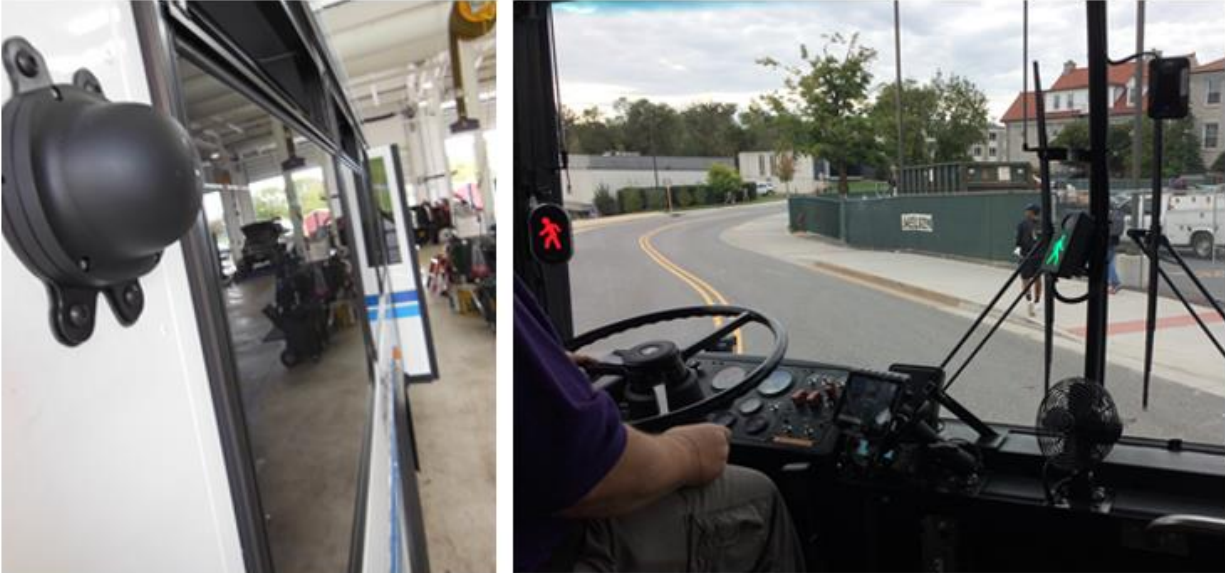
Figure 1. Right Rear Collision Avoidance Warning System (CAWS) Camera (Left) and Operator’s Compartment With Left Alert Display Illuminated Red, Center Alert Display Illuminated Green, and Center Camera Mounted Near Parked Wiper (Right)
