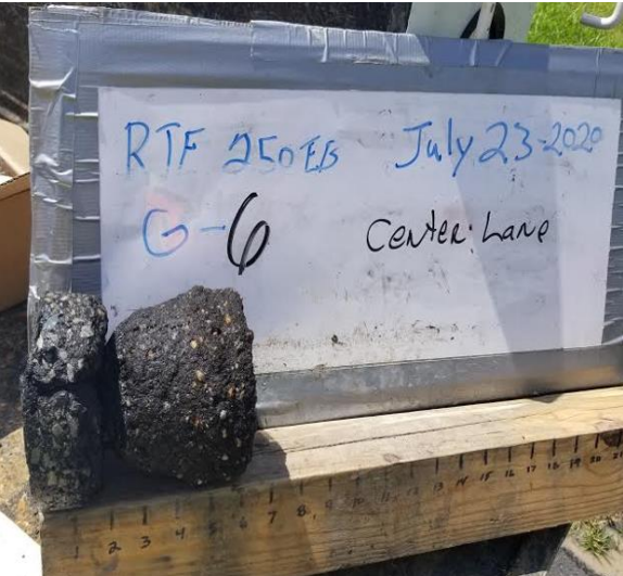
Figure C2. Core Photographs From Rte. 250
