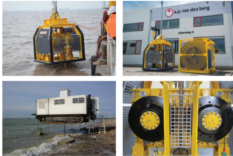
Figure 1.15 Near-shore and off-shore CPT rigs (courtesy of A.P. van den Berg, n.d).
