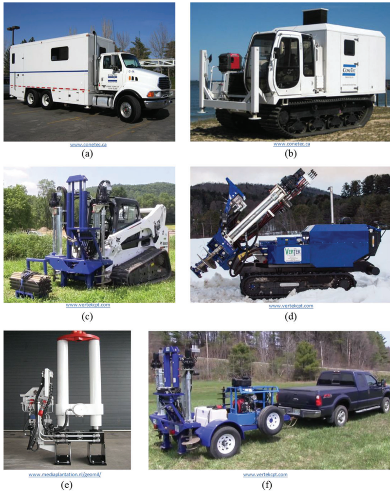
Figure 1.14 Cone penetrometer rigs: (a) truck-mounted rig (ConeTec Inc., n.d.), (b) track-mounted CPT rig with closed cabin for data acquisition and recording (ConeTec Inc., n.d.), (c) and (d) front-mounted CPT rigs with ground anchors (Vertek, n.d.), (e) portable CPT rig (Geomil Equipment B.V., n.d.), and (f) towed CPT rig (Vertek, n.d.).
