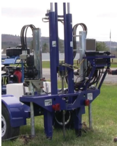
Figure 1.12 CPT hydraulic ram, clamping, and thrust system (courtesy of Vertek, n.d).
