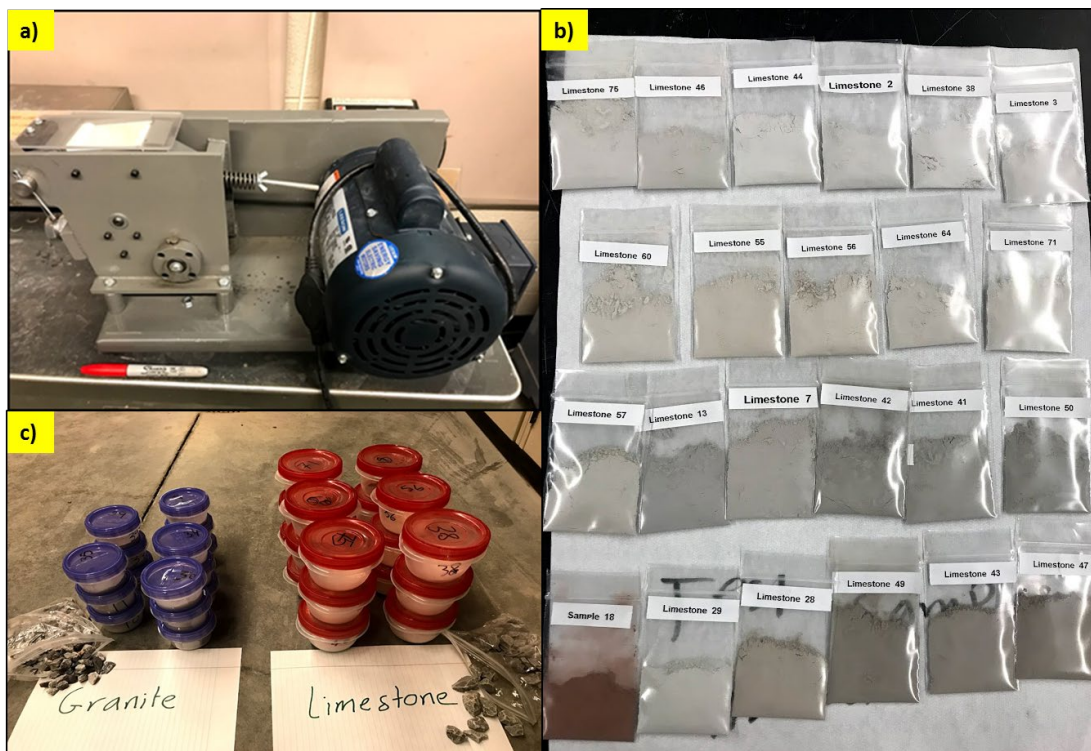
Figure 3.4 Aggregate preparation for chemical and XRD testing: (a) Mini-jaw crusher, (b & c) aggregate powder samples for testing
