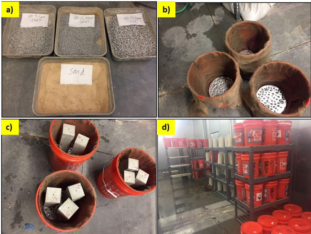
Figure 3.2 Aggregate testing per ASTM C1293: (a) aggregate preparation in standard gradation, (b and c) conditioning containers, (d) conditioning in curing room at 38°C (100°F) for one year for evaluating aggregate reactivity and two years for evaluating mitigation alternatives.
