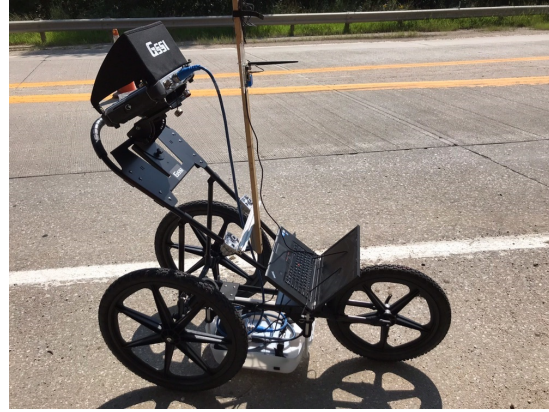
(b) GPR system on a survey cart
