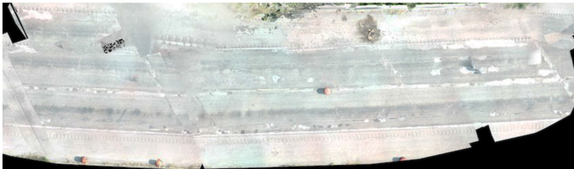
(a) Stitched UAV image collected on asphalt overlaid concrete deck
