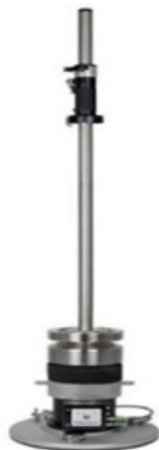
Figure 2 - Light Weight Deflectometer (LWD) measures deflection by dropping a weight by hand.
