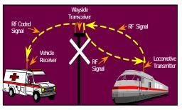
Figure 3. Three-point VPAS Concept
