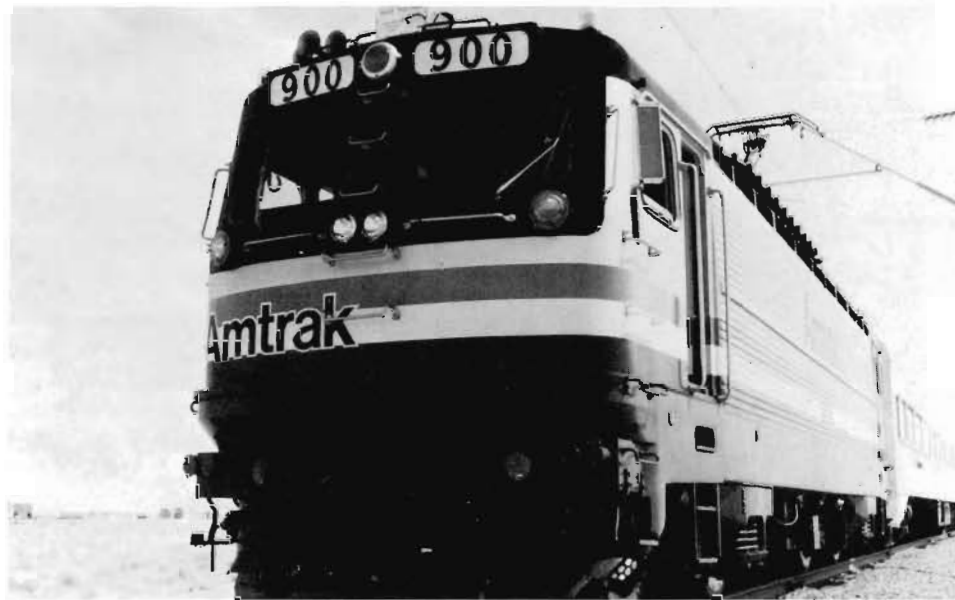
RTT ELECTRIFICATION – AMTRAK AEM-7 LOCOMOTIVE STANDS READY ON RTT TO BEGIN TEST
