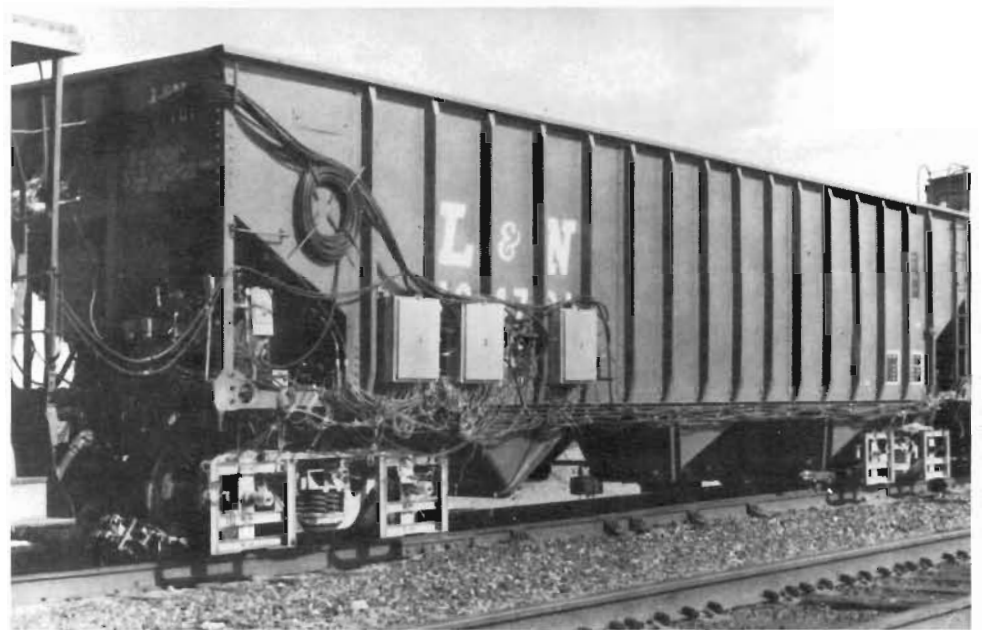
FREIGHT CAR-DYNAMIC TESTING VEHICLE
