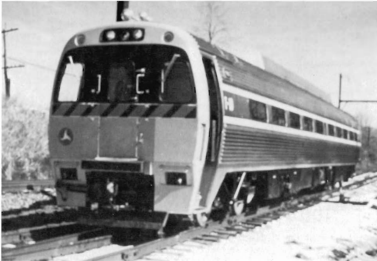
BUDD SPV-2000 DESIGNATED FRA T-10, THE FIRST SELF-PROPELLED ATIP VEHICLE, WILL STREAMLINE THE TRACK GEOMETRY MEASUREMENT PROCESS WHILE ADDING A REDUNDANT DATA PROCESSING SYSTEM AND ENHANCING SYSTEM RELIABILITY.
