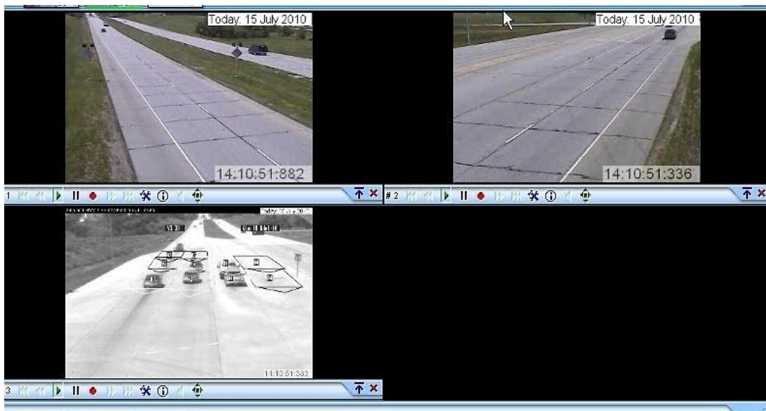
Figure 3.7 Display of recorded vehicular movement through data collection site
