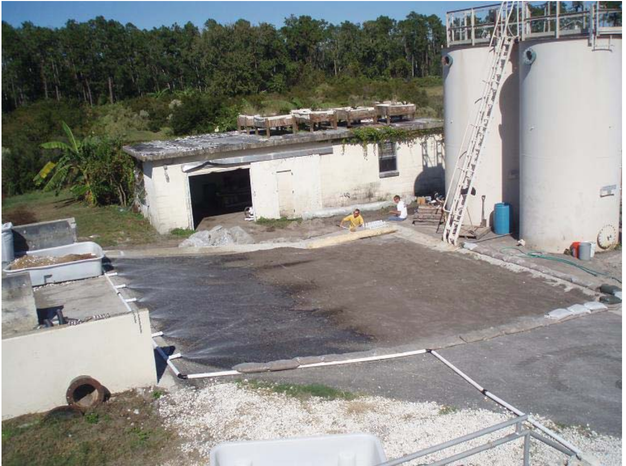
Figure 126: Curb inlet test field with sheet flow simulator
