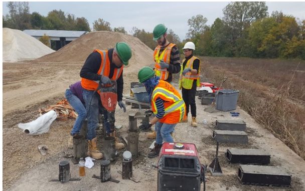
Figure 14. Sampling of concrete
