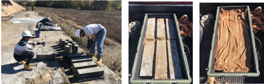
Figure 18. Demolding and transportation of samples
