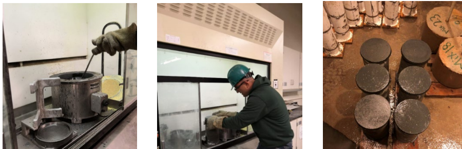
Figure 19. Demolding and transportation of samples
