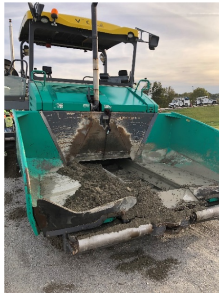
Figure 10. Loading process of the slip-form paving
