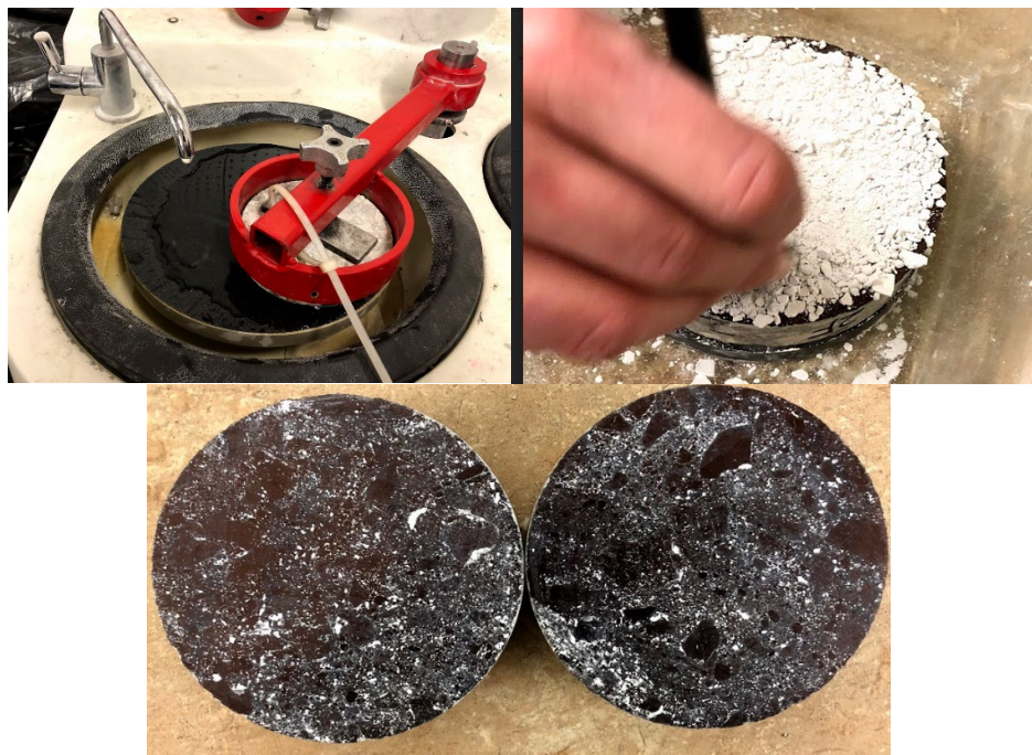
Figure 27. Sample preparation for air-void system analysis
