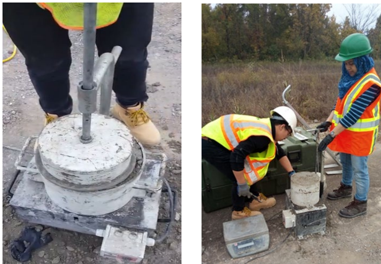
Figure 15. Vebe test apparatus for determining consistency/density of fresh CCP
