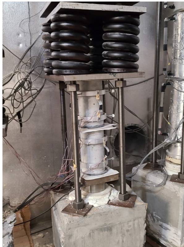
Figure 3-11. Concrete creep test setup
