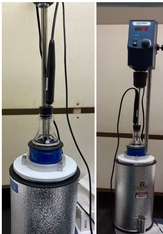
Figure 3.14 Complete arrangement of the equipment used in freezing point determination.
