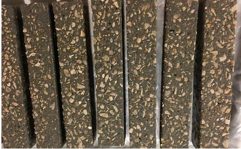
Figure 3.33 PCC beams after F-T cycles
