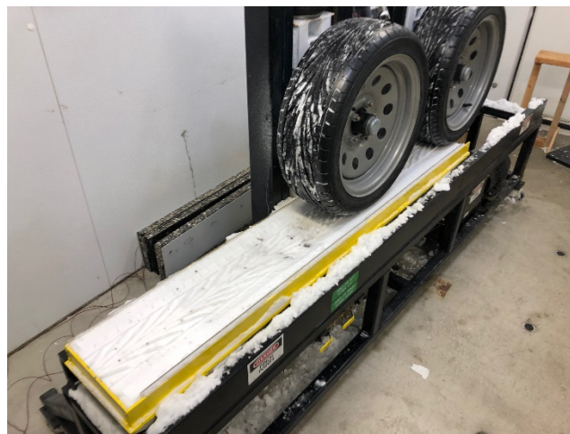
Figure 3.17 Automated trafficking machine used in this research.
