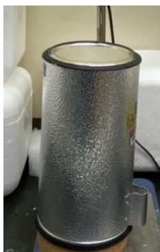
Figure 3.10 Dewar flask (2100 mL, silvered and evacuated) to be used for cooling bath
