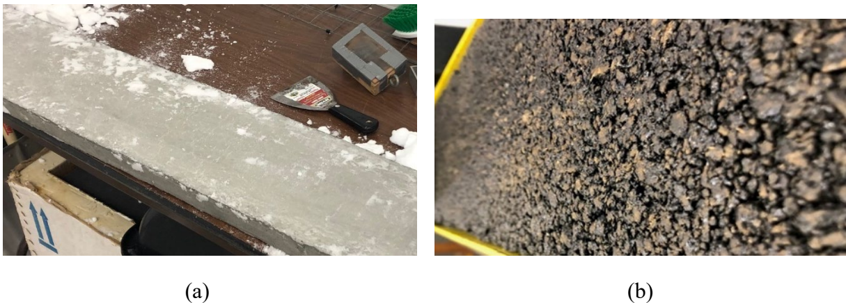
Figure 3.16 Examples of test samples for different types of pavements: (a) concrete pavement, (b) asphalt pavement.
