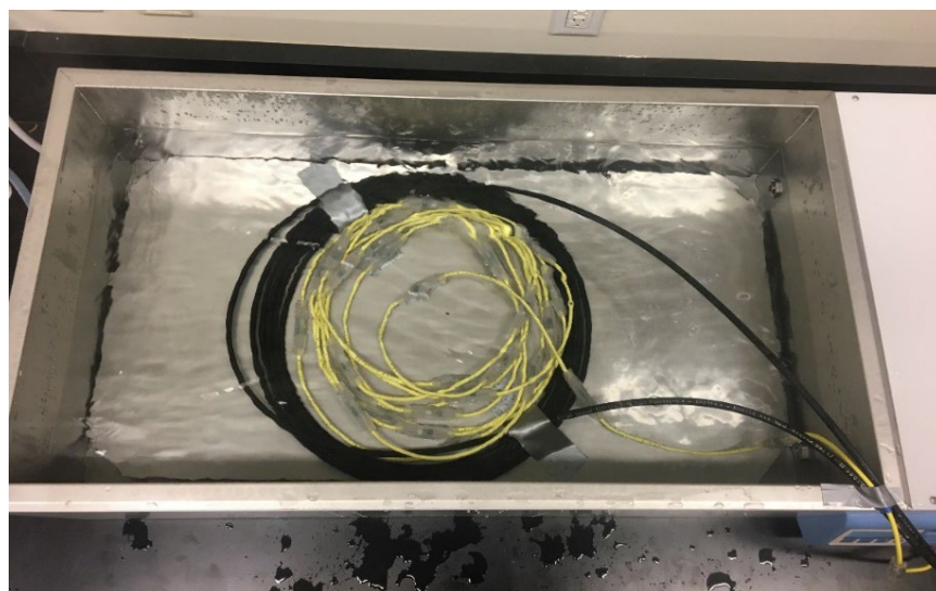
Figure 3-2: Photograph of the cable configuration within the water bath.
