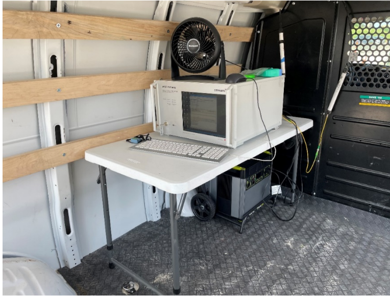
Figure 4-22: Photograph of the fiber optic analyzer setup in the rear of the cargo van.
