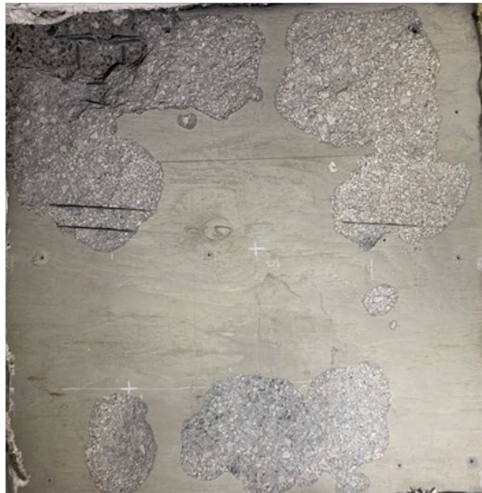
Figure 5.30 Heated surfaces of (a) TS1, (b) TS 2, (c) TS 3, and (d) TS 4 after fire tests, showing cracked and spalled concrete
