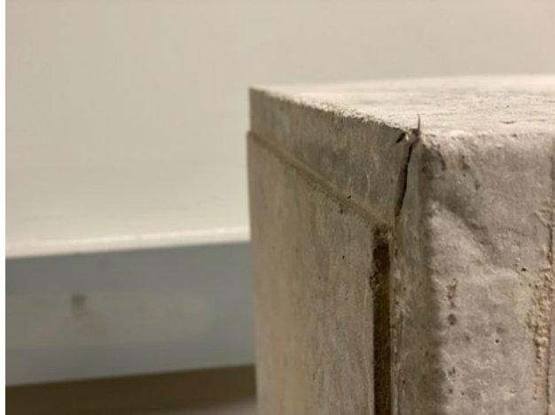
Figure 4.2 Side view of the specimen showing a setback on the front (heated) side of a specimen
