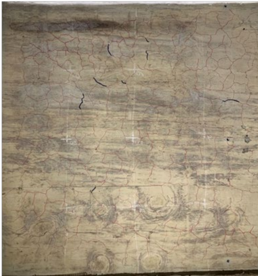
Figure 5.30 Heated surfaces of (a) TS1, (b) TS 2, (c) TS 3, and (d) TS 4 after fire tests, showing cracked and spalled concrete
