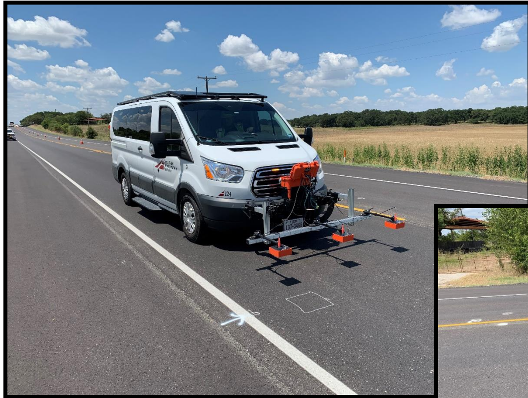
Survey with GPR
