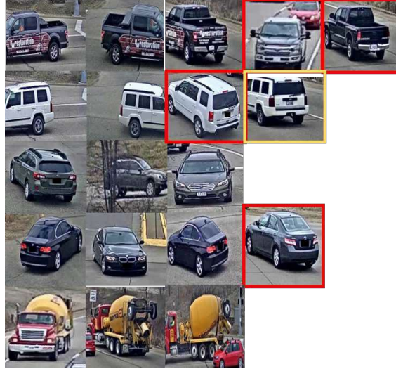
Figure 10: Visualization results of MTMC on five different kinds of vehicles. Each image represents a tracklet and each line represents these tracks from different camera views are classified by MTMC to be from the same vehicle. Yellow box represents false negative and red box represents false positive.
