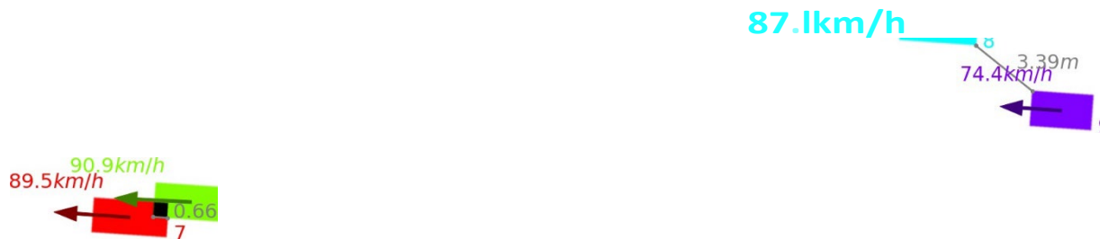
Figure 4. Danger recognition: four vehicles in a sample prediction of the road plane, with vehicle IDs at the bottom right and speeds at the top left. Distances are shown for nearing vehicles, and danger area is shown in black at the overlap of vehicle 7 and 10.
