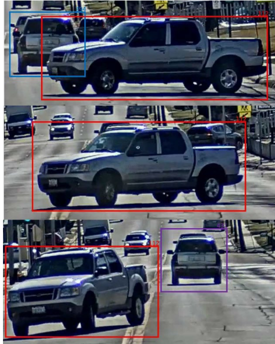
Figure 3: Different from SOT, tracking ID in MOT usually change due to overlapping. Thus, rules, filters or smoothing functions are needed.
