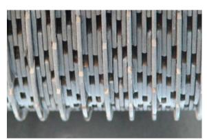
(c) Figure 7. Heads of (a) grinding, (b) grooving, and (c) NGCS [34].
