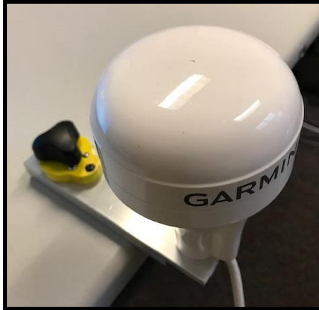
Figure 3. GPS Antenna Mounting.
