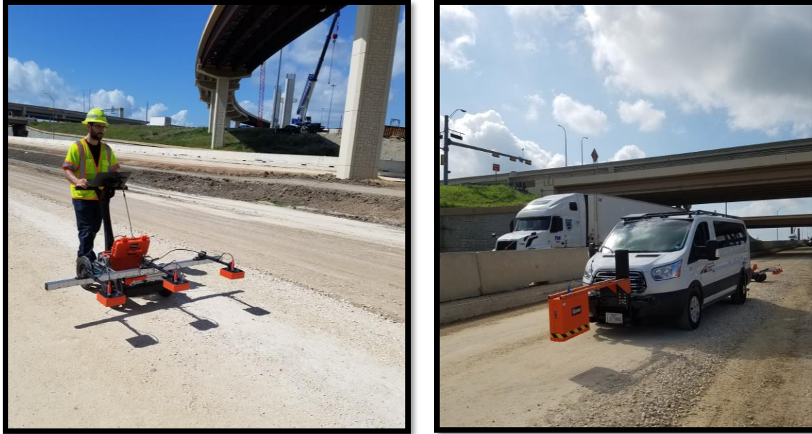
Figure 11. GPR Collection on SH 130 for Mechanics-Based Models.
