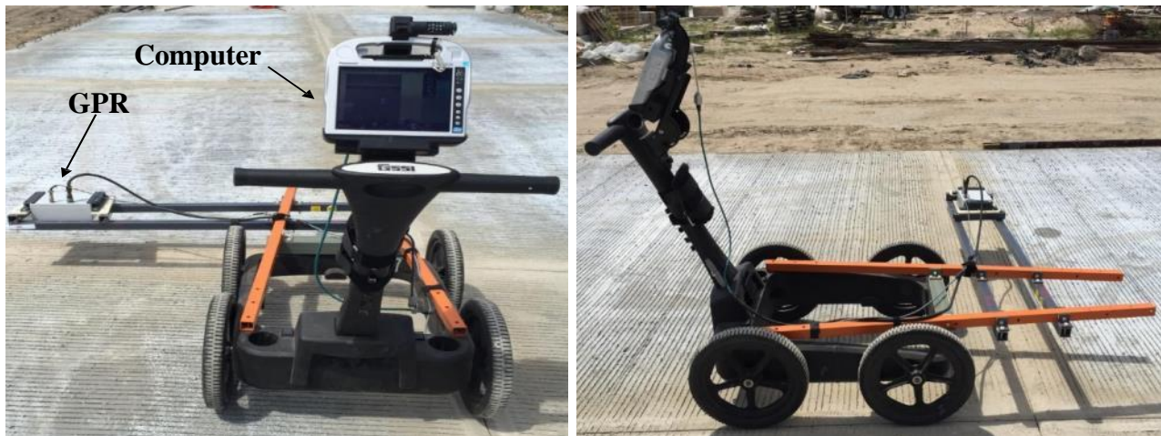
Figure 121. GPR used for concrete EI Measurement.
