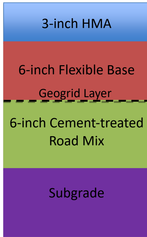
Figure 32. Structures of Identified Pavement Sections in SH 21.
