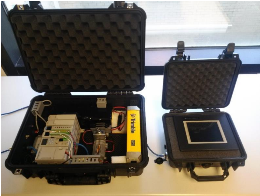
Figure 63. Final Hardware version (small nominal 6” HMI on right, PLC, battery, signal conditioning, GPS unit and on/off switch in left case).
