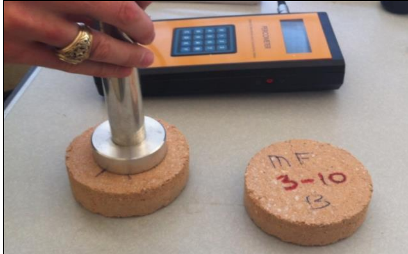
Figure 12. Measurement of Dielectric Constant of Flexible Base Using Percometer.
