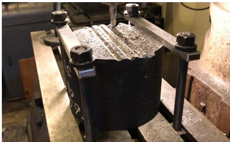
Figure 3-12. Drilling machine used for artificial milled surfaces.
