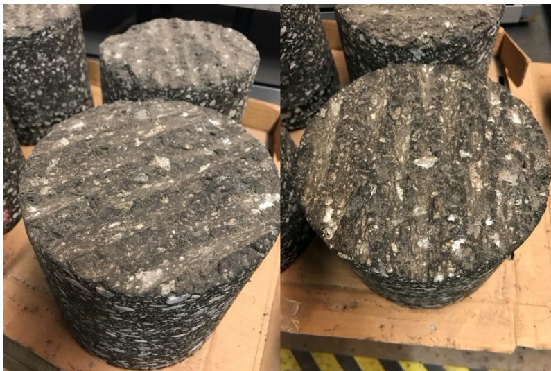
Figure 3-7. Milled surface field cores.
