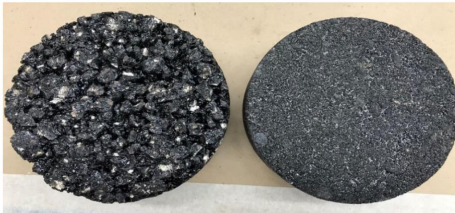
Figure A3. High texture (left) and low texture (right) mixtures (Bahia et al. 2019).
