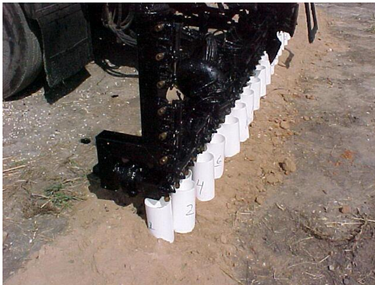
Figure 7-16. Calibrating distributor volumetrically (courtesy: http://onlinemanuals.txdot.gov/txdotmanuals/scm/asphalt_distributor.htm#i1007776 ).
