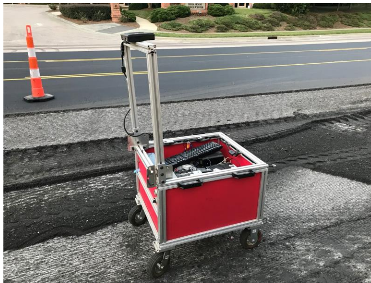
Figure 3-16. 3-D laser profiler on Maynard Rd., Cary, NC.
