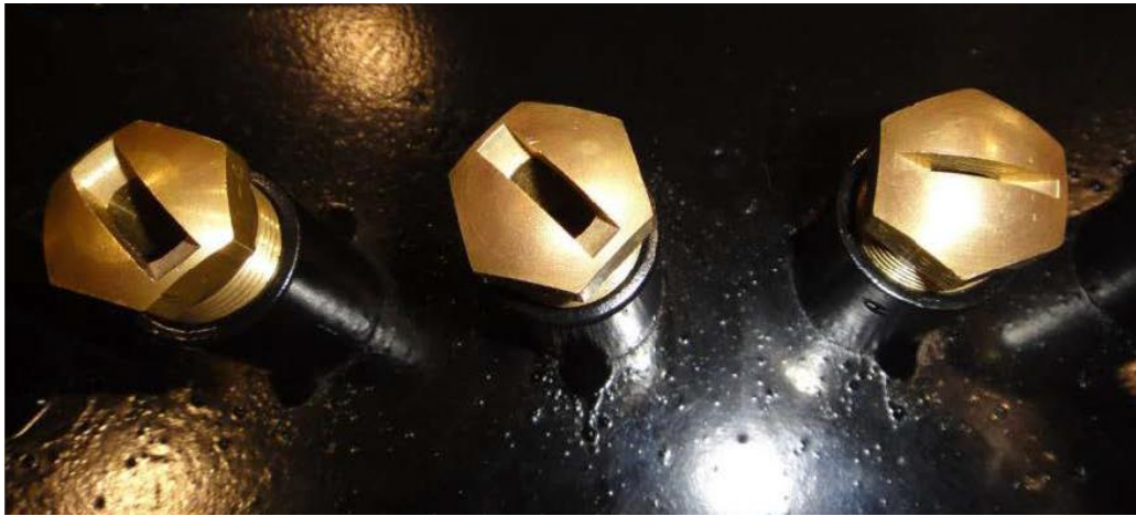
Figure 7-8. Examples of different nozzle sizes for different application rates (FHWA 2016).
