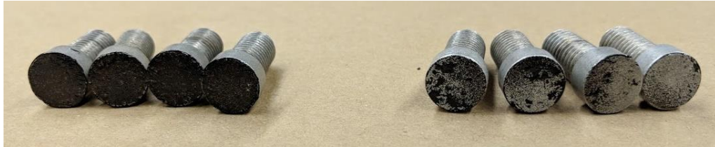
Figure 5-28. Failure mode of CRS-2 (left) compared to CRS-1h (right) at 5°C.
