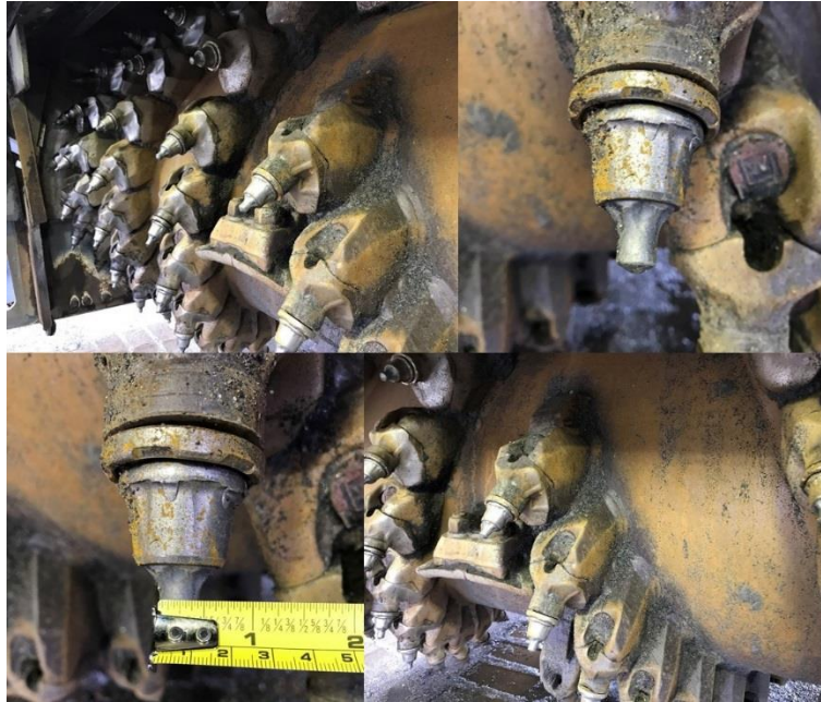
Figure 3-11. Milling machine: teeth details.
