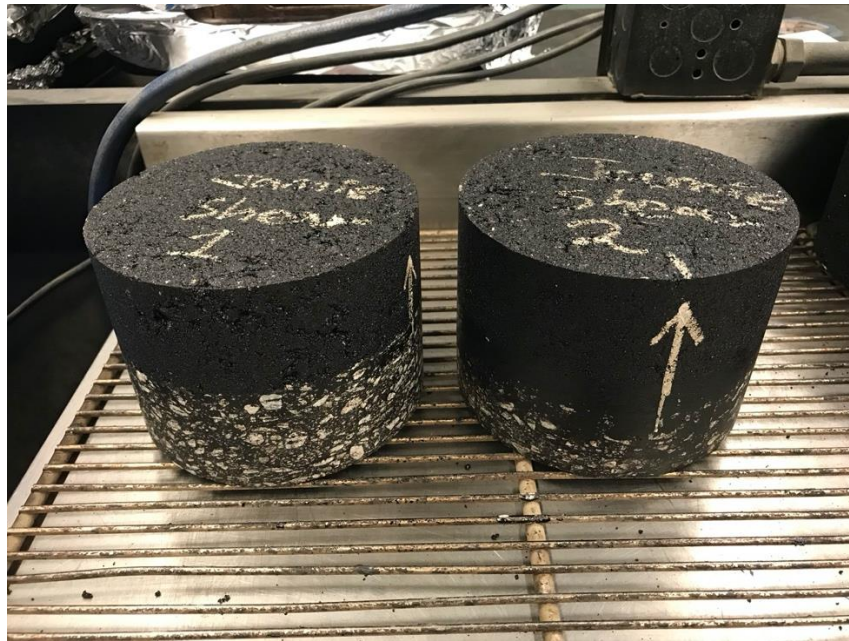
Figure 3-8. Two milled surface gyratory-compacted specimens.
