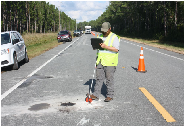
Figure 3-14. PCI Cracking Survey Process
