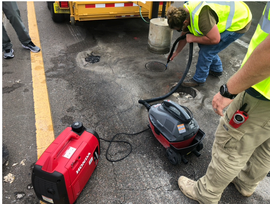
Figure 3-20. Partial-Depth Wet-Coring and Vacuuming of 12-in Diameter AC Samples Prior to Dry Coring
