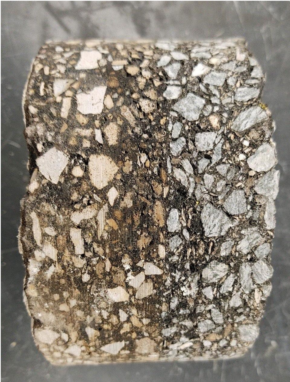
Figure 4-89. Close-up of Air Voids at US 17 Worm Core Layer Interface
