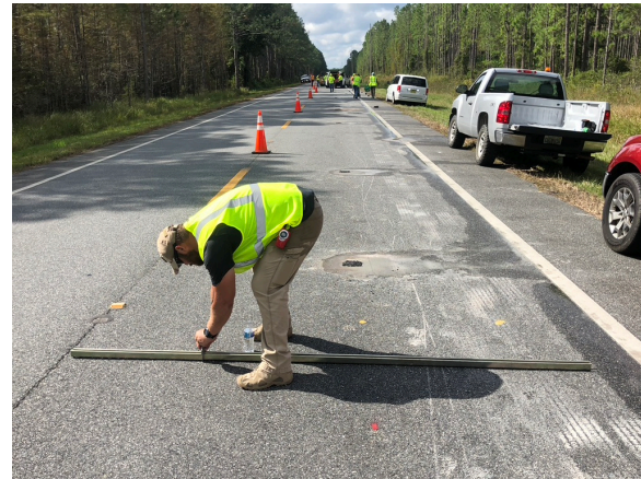
Figure 3-15. PCI Rutting Survey Process
