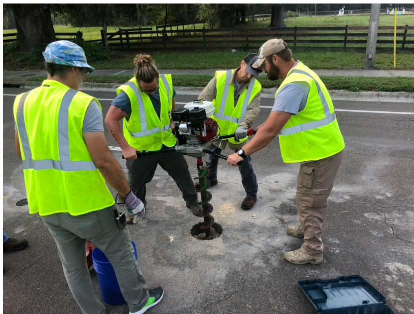
Figure 3-21. Sampling Base, Subgrade, and Embankment Materials
