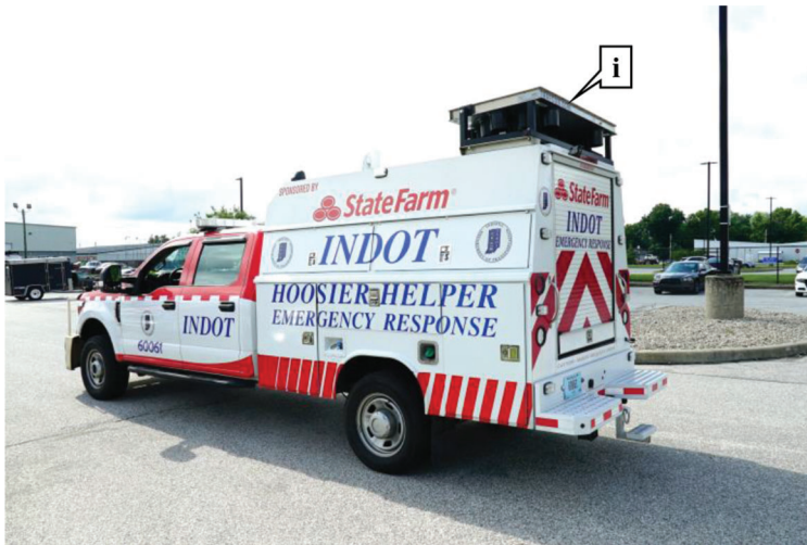
Figure 1.2 Example of a Hoosier Helper with an integrated sign (callout i) and markings on the back.
