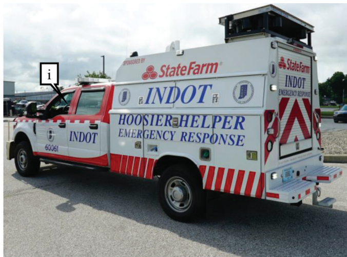
(a) Hoosier Helper with installed HAAS Alert device at Indianapolis TMC
