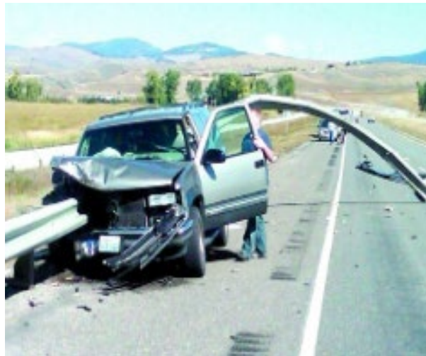
Figure 1.4: An Example of a Vehicle Crash with a Guardrail Blunt-End Source: Glennon (2012)
