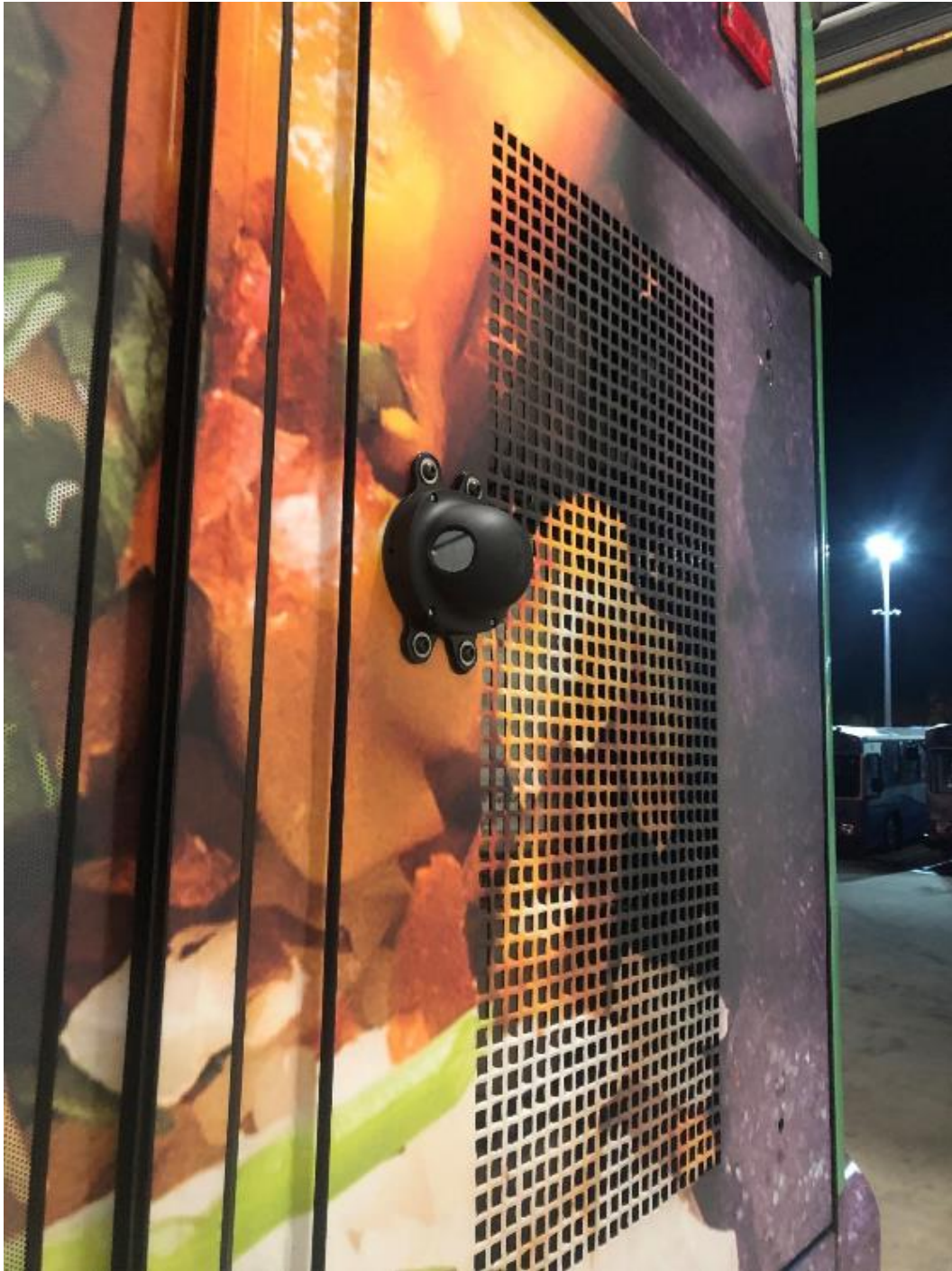
Figure D-4 – Street-side rear sensor placement
