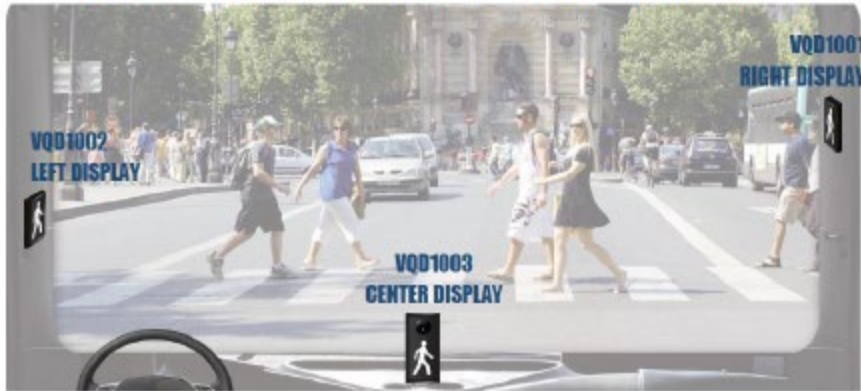
Displays Mounted in line with the driver mirrors, facing the driver
