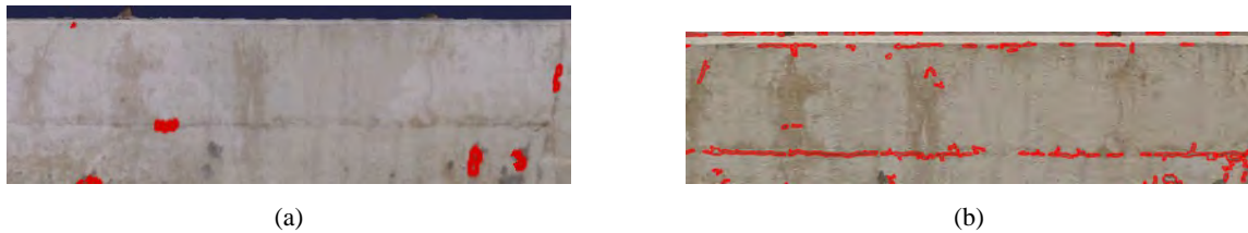
Figure 4.8 Comparison of defect detection using: (a) texture mapping technique, and (b) the originally proposed technique
