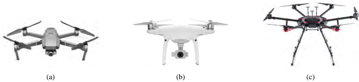
Figure 2.2 UAV platforms tested: (a) DJI Mavic 2 Zoom - wingspan: 1.05 feet [32], (b) DJI Phantom 4 Pro - wingspan: 1.15 feet [33], and (c) DJI Matrice 600 Pro - wingspan: 5.47 feet [34]
