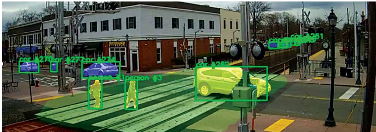
Example of video processing output showing pedestrians and vehicles traversing a grade crossing at Ramsey, NJ. Source: U.S. DOT Volpe Center
