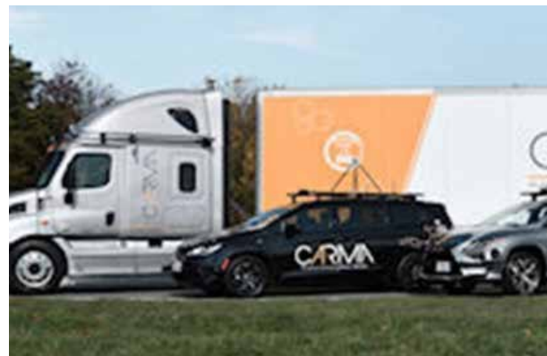
Passenger vehicles and a heavy truck in the Cooperative Automation Research Mobility Applications (CARMASM) research fleet. Developed by FHWA, CARMA is open-source software that supports cooperative driving automation. Source: FHWA
