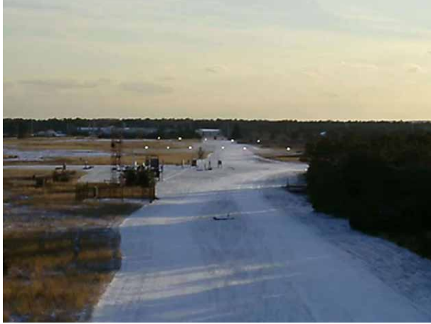
LED lamps for airport lighting are seen side-by-side with their incandescent counterparts at the Aviation Weather Research Facility. Source: U.S. DOT Volpe Center
