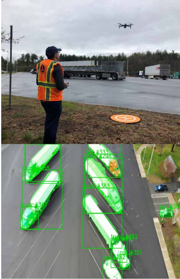
The Truck-Parking-Using-Drones VIA team explored the use of an autonomous drone equipped with machine learning and AI to inform truckers of available parking and reduce dangerous parking on ramps. Source: U.S. DOT Volpe Center
