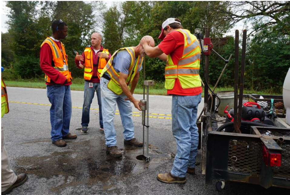
Figure 4. Dynamic cone penetrometer testing on NC 96.
