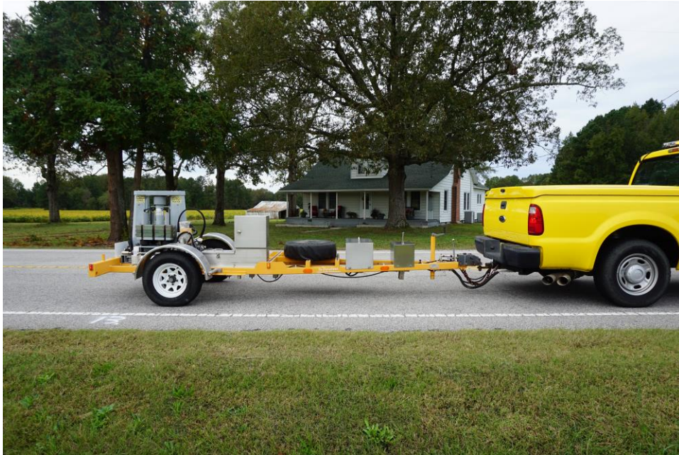
Figure 3. Falling weight deflectometer testing on NC 96.
