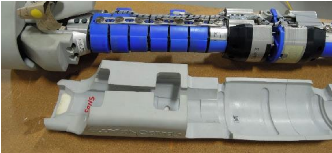
Figure 4. A view of the aPLI next to its one-piece molded flesh system.
