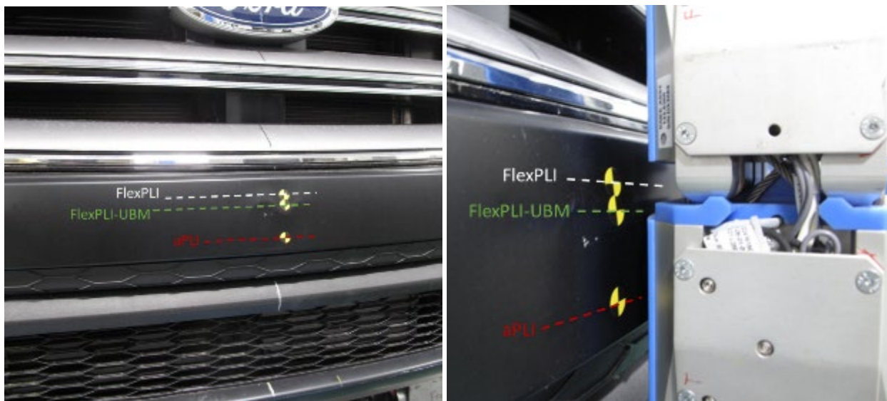
Figure 20. Knee centerline impact locations for the FlexPLI, FlexPLI-UBM, and aPLI.
