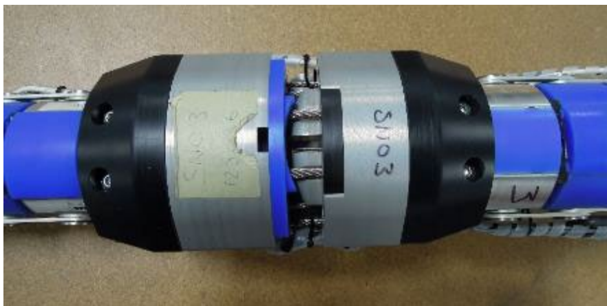
Figure 6. Rounded knee block of the aPLI to improve legform response in oblique impacts. Additionally, the orientation of the knee ligaments was modified to be vertical to improve biofidelity (Figure 7).
