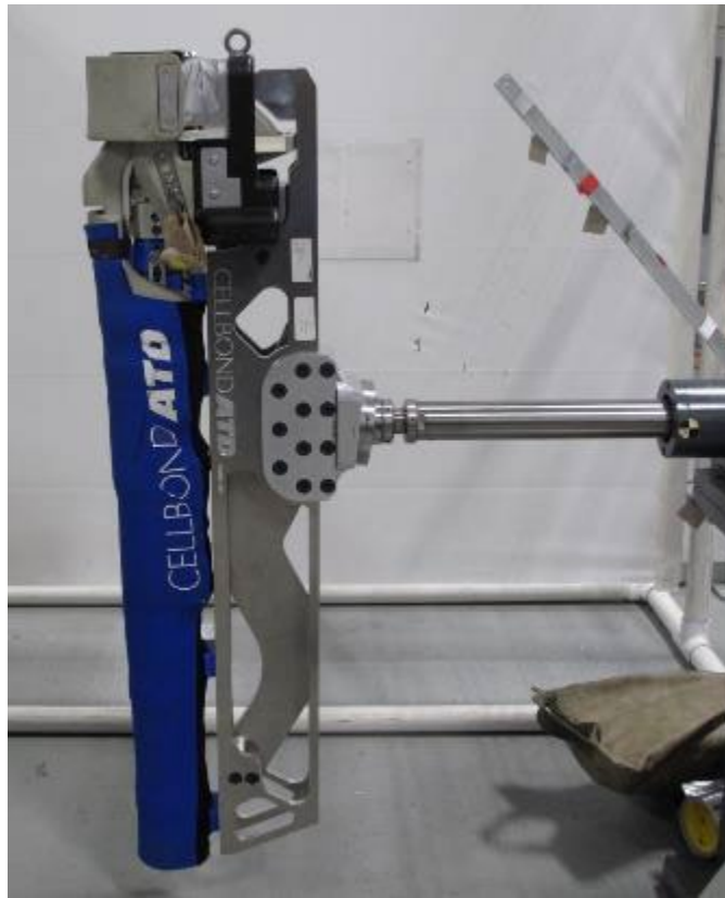
Figure 11. View of the aPLI carriage attached to VRTC's launch system.
