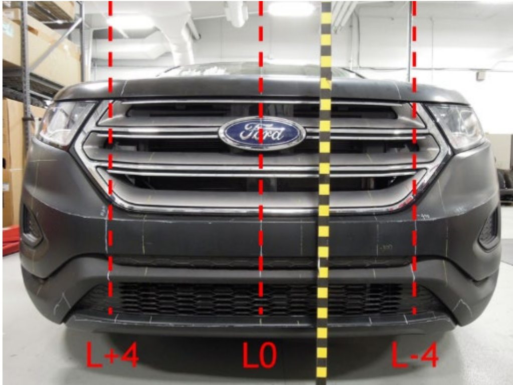
Figure 9. Frontal view of the 2016 Ford Edge shown with legform impact locations.
