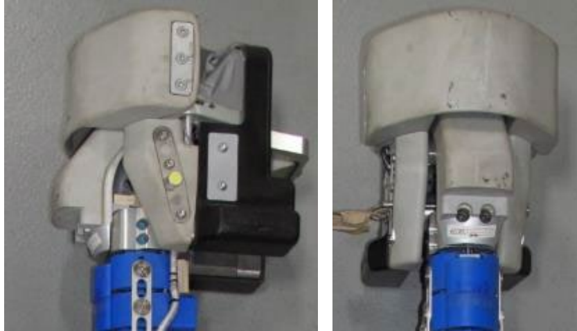
Figure 3. View of the SUBP: (Left) Anterior view; (Right) Lateral/struck-side view.
