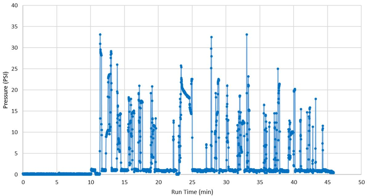
**Figure 22. Brake pressure (left rear brake): Local**
