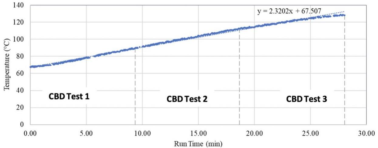
**Figure 8. Brake pad temperature (right rear brake): CBD**
