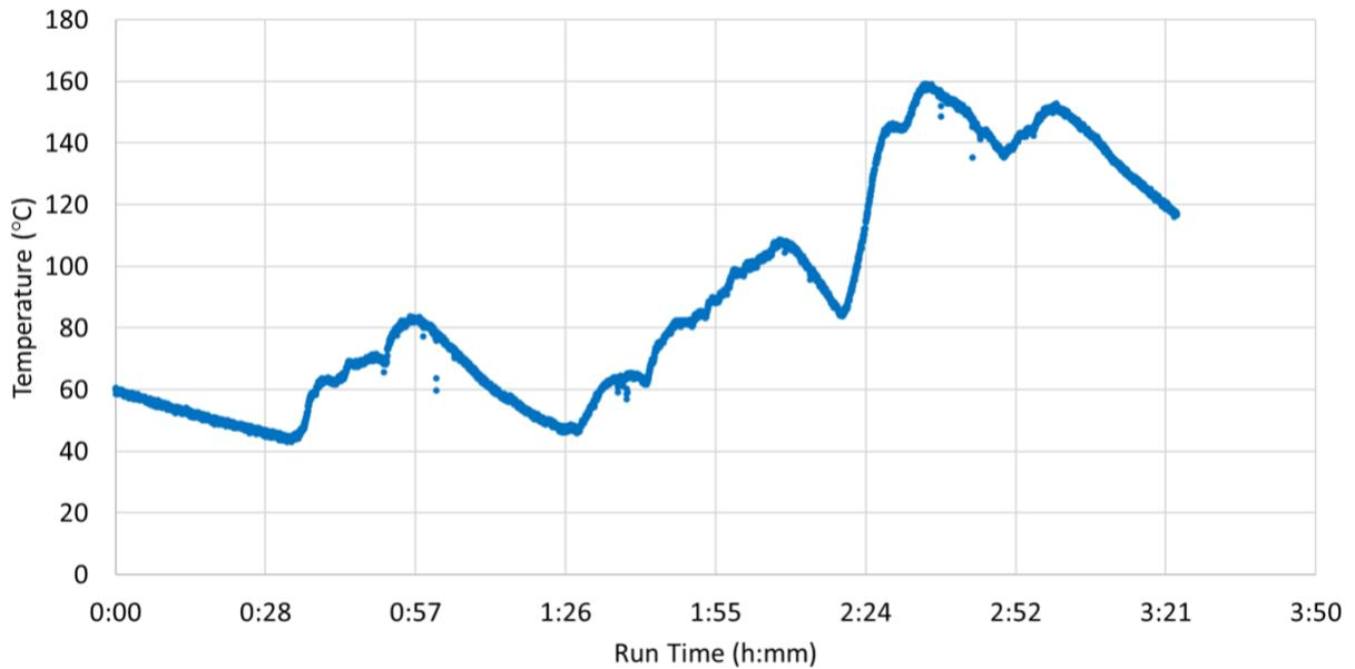
**Figure 27. Brake temperature (left rear brake): Freeway route**
