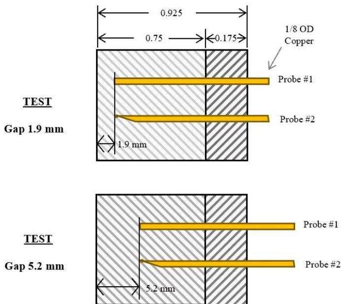
**Figure 34. Cross section diagram of thermocouple installation**
