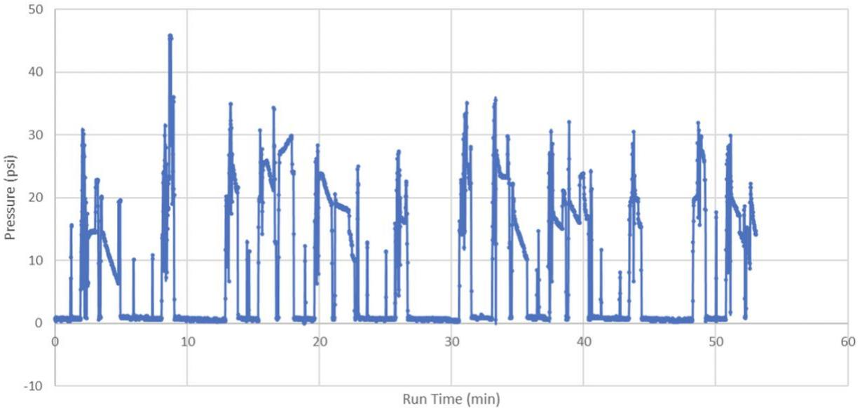
**Figure 16. Brake pressure (right rear brake): UDDS**
