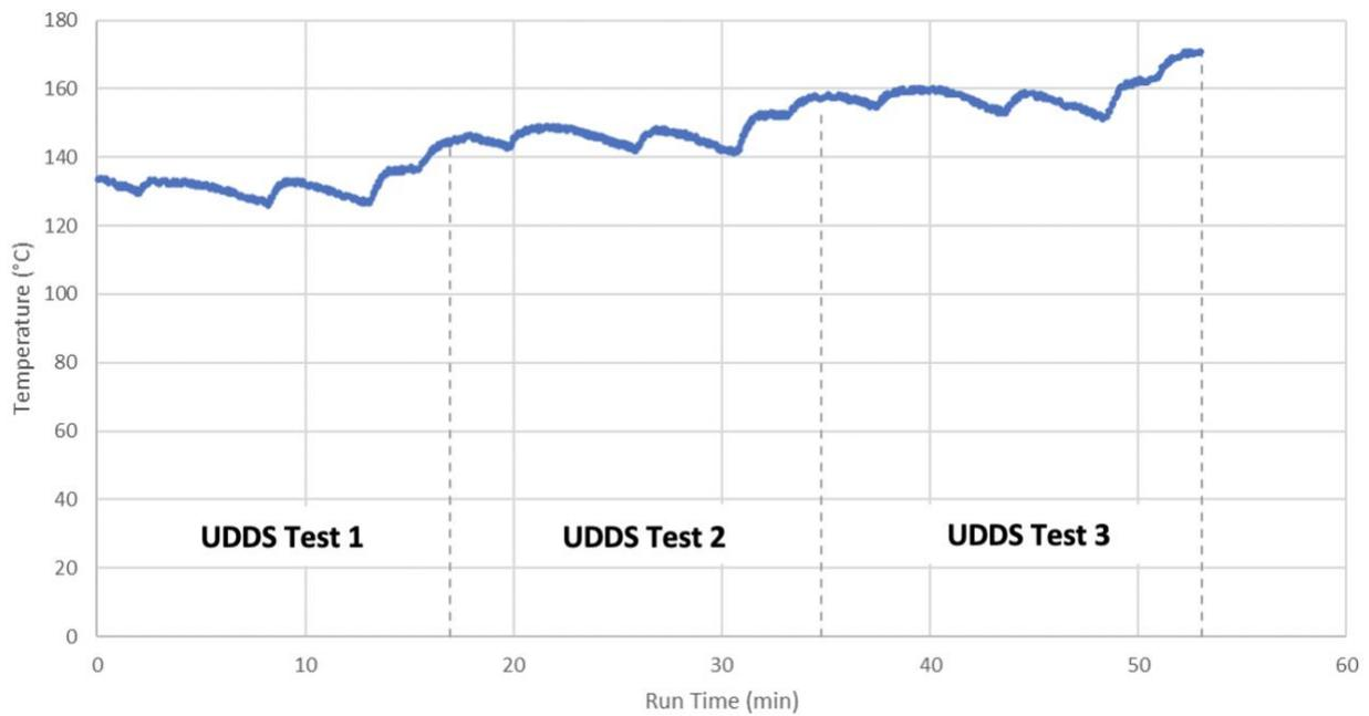
**Figure 15. Brake pad temperature (left rear brake): UDDS**
