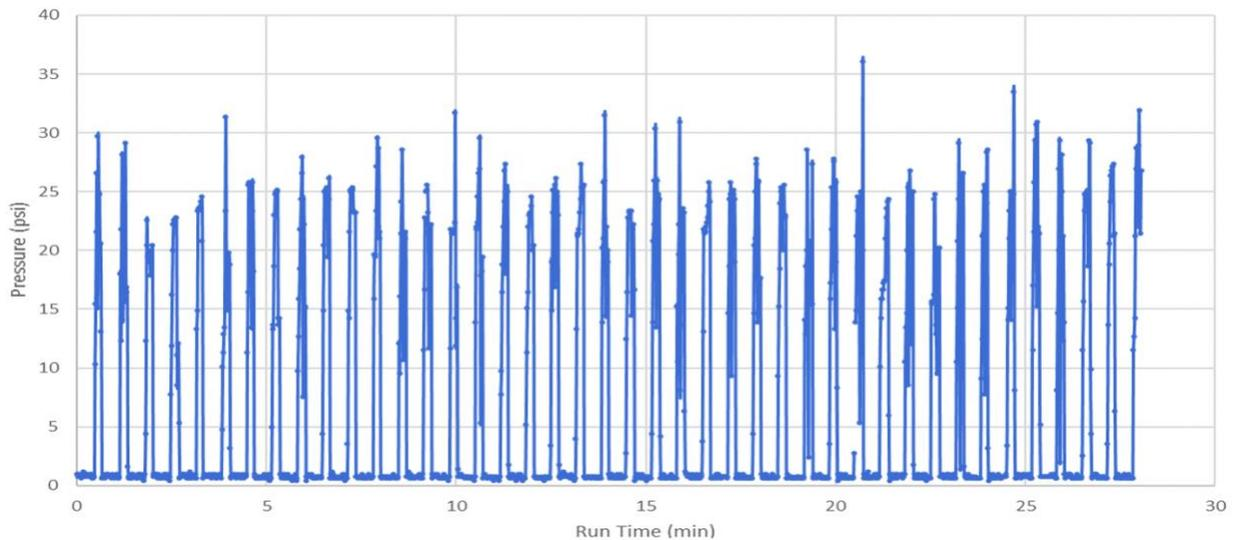
**Figure 9. Brake pad pressure (right rear brake): CBD**
