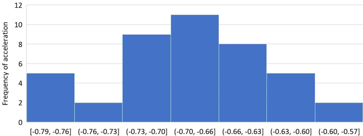
**Figure 11. Average acceleration (m/s<sup>2</sup>) histogram for braking activity: CBD**
