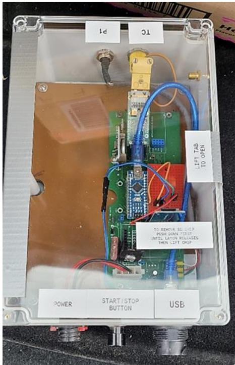
**Figure 4. Brake logger with temperature and pressure inputs**
