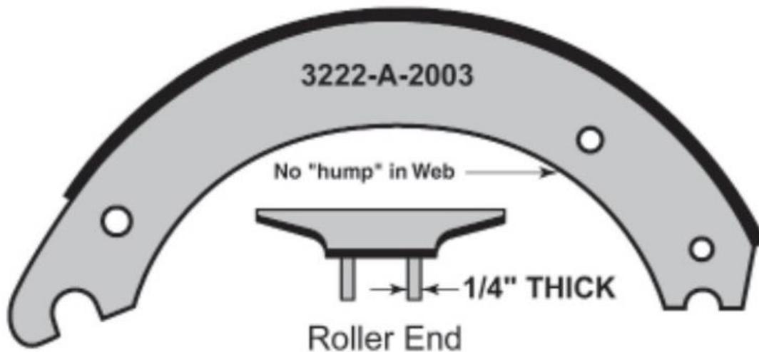
Figure 2. 16-1/2" x 8-5/8" Meritor Q Plus Brake shoe. (Meritor 2018)
