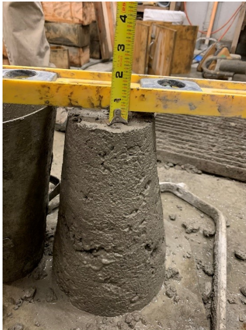
Figure A.62: Result from slump testing (Mixture 22)
