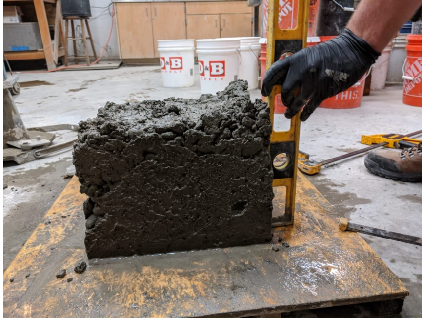
Figure A.55: Surface-void profile for one of the sides of box test specimen (Mixture 20)
