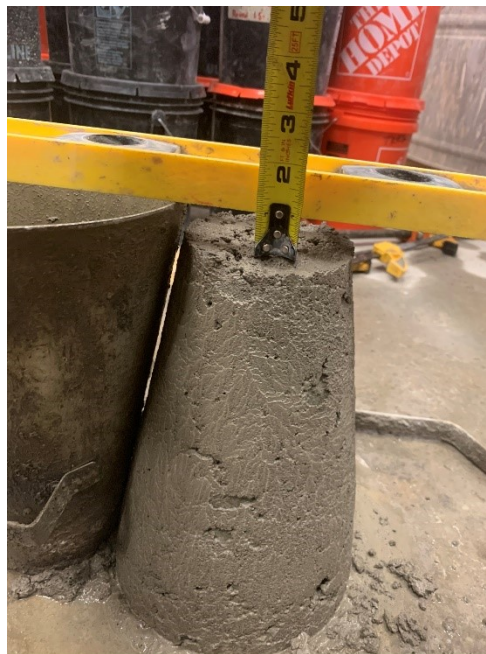
Figure A.28: Result from slump testing (Mixture 8)
