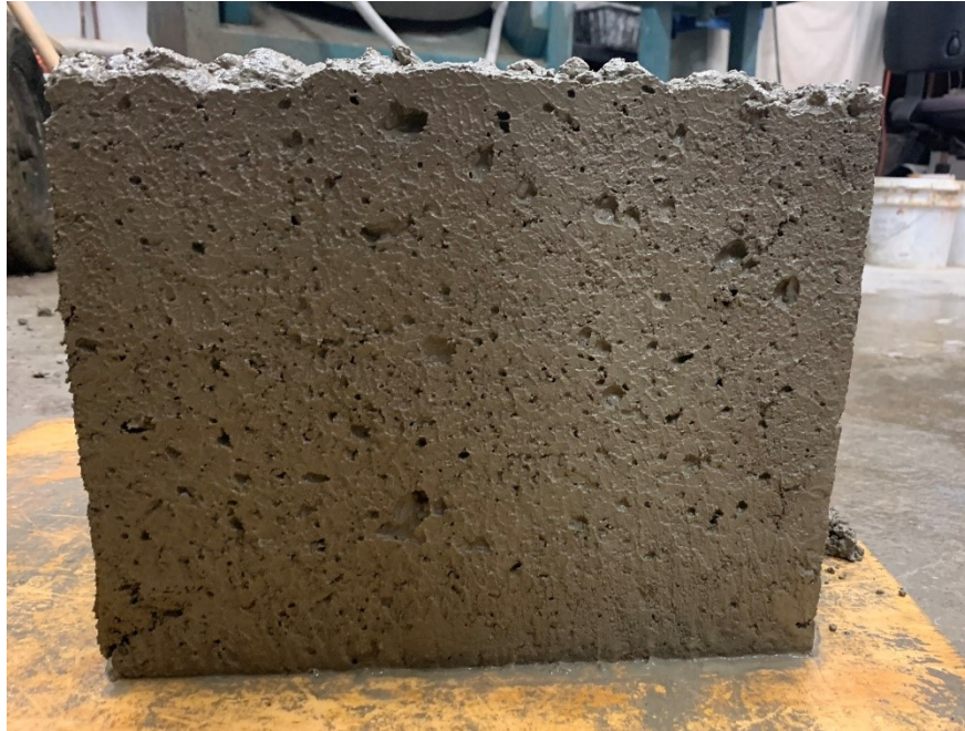
Figure A.42: Surface-void profile for one of the sides of box test specimen (Mixture 13)
