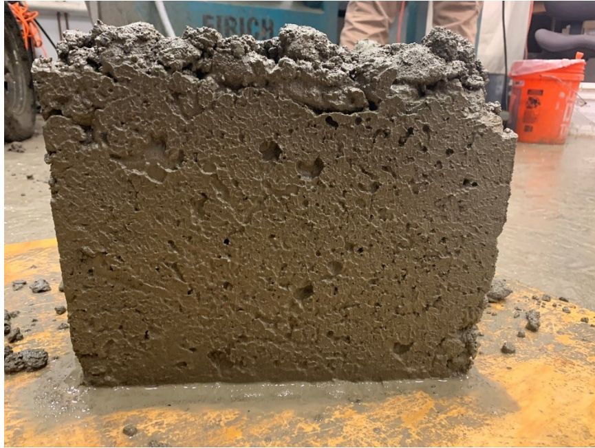
Figure A.51: Surface-void profile for one of the sides of box test specimen (Mixture 16)
