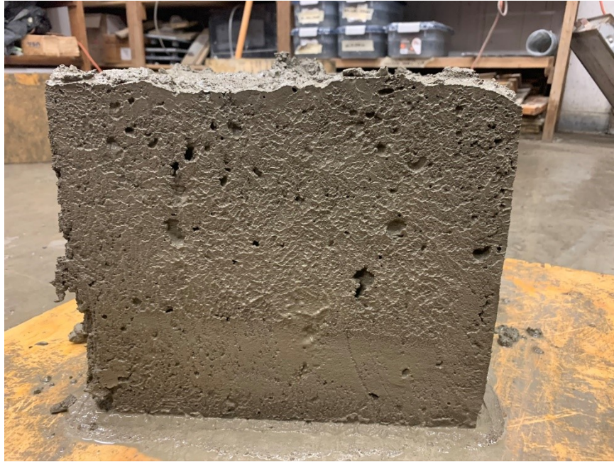
Figure A.27: Surface-void profile for one of the sides of box test specimen (Mixture 8)
