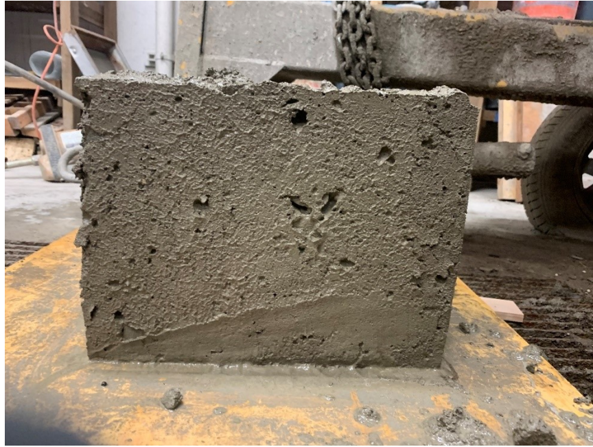
Figure A.5: Surface-void profile for one of the sides of box test specimen (Mixture 2)
