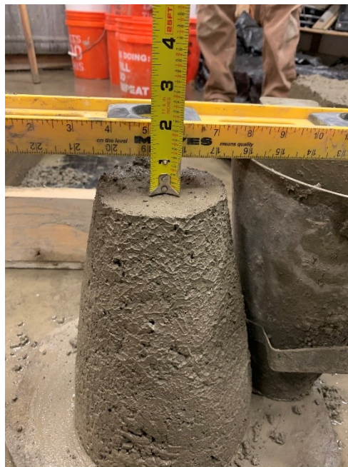
Figure A.25: Result from slump testing (Mixture 7)
