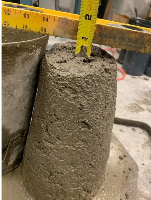
Figure A.18: Result from slump testing (Mixture 5)
