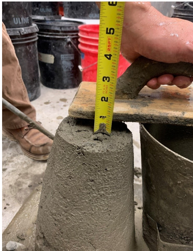
Figure A.6: Result from slump testing (Mixture 2)
