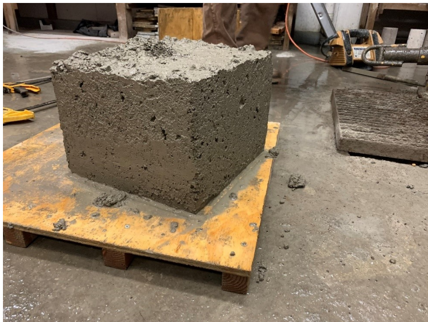
Figure A.17: Overview of box test specimen (Mixture 5)
