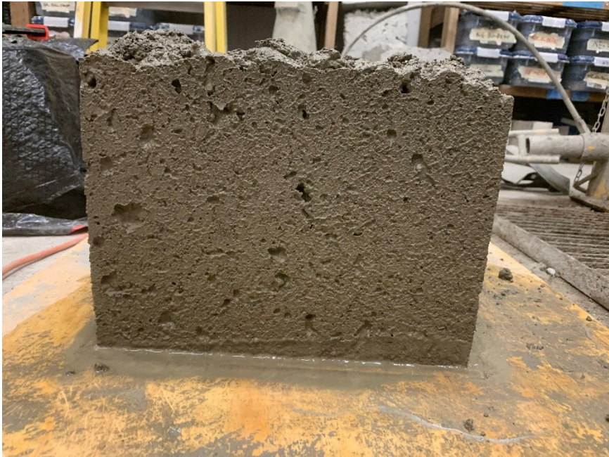
Figure A.1: Surface-void profile for one of the sides of box test specimen (Mixture 1)
