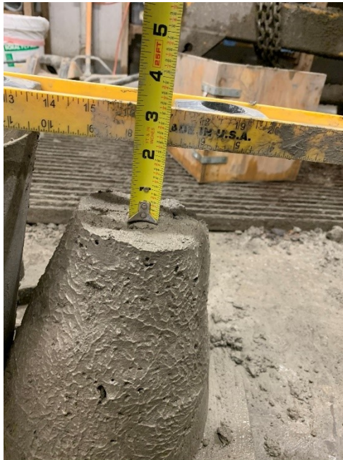
Figure A.58: Result from slump testing (Mixture 23)
