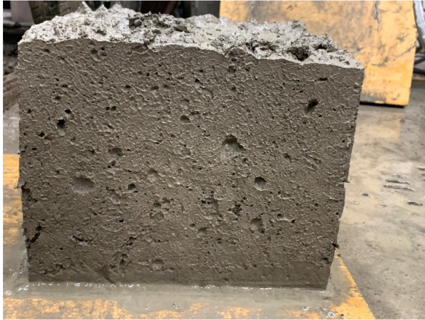
Figure A.8: Surface-void profile for one of the sides of box test specimen (Mixture 3)
