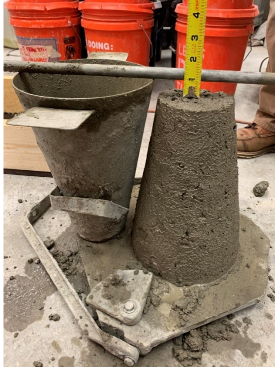
Figure A.3: Result from slump testing (Mixture 1)
