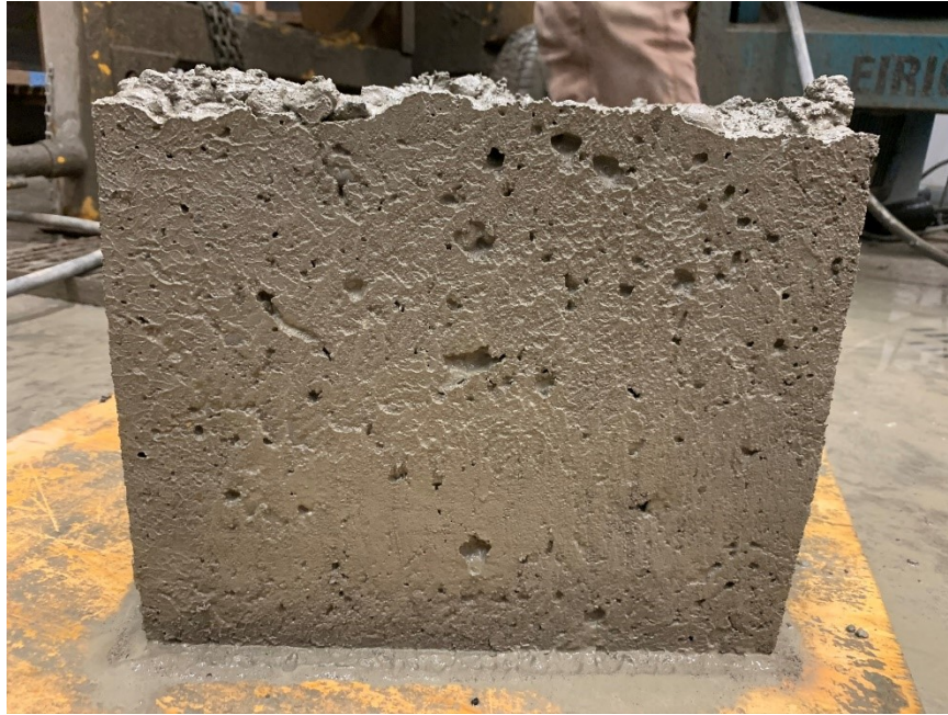
Figure A.36: Surface-void profile for one of the sides of box test specimen (Mixture 11)
