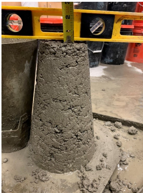
Figure A.45: Result from slump testing (Mixture 14)
