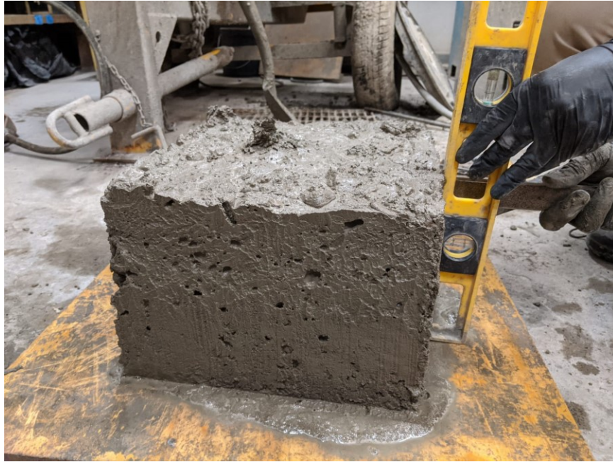
Figure A.60: Surface-void profile for one of the sides of box test specimen (Mixture 21)
