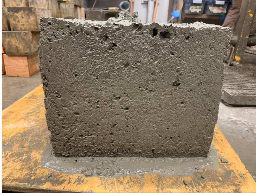
Figure A.47: Surface-void profile for one of the sides of box test specimen (Mixture 15)
