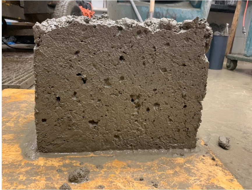
Figure A.49: Surface-void profile for one of the sides of box test specimen (Mixture 17)
