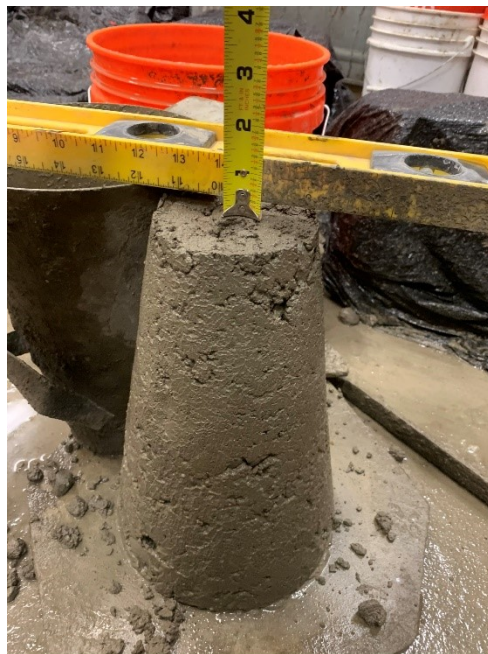
Figure A.50: Result from slump testing (Mixture 17)
