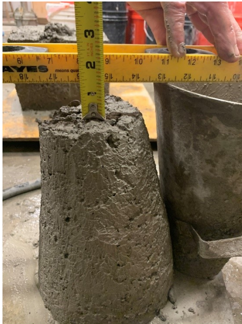
Figure A.48: Result from slump testing (Mixture 15)
