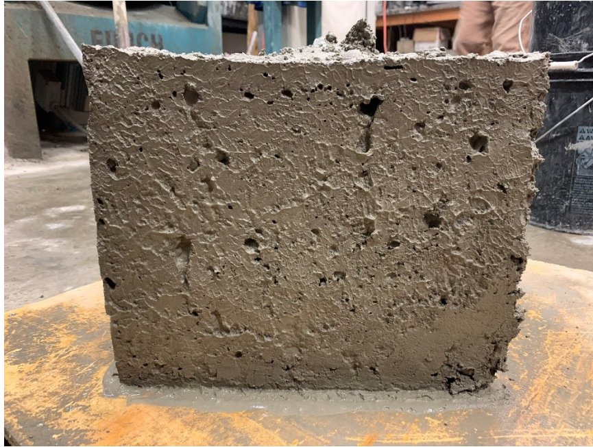
Figure A.39: Surface-void profile for one of the sides of box test specimen (Mixture 12)
