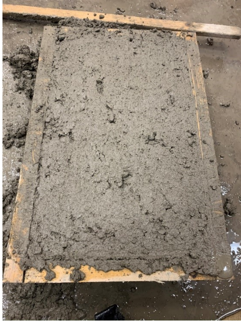
Figure A.26: Concrete finished surface after screeding and troweling (Mixture 7)
