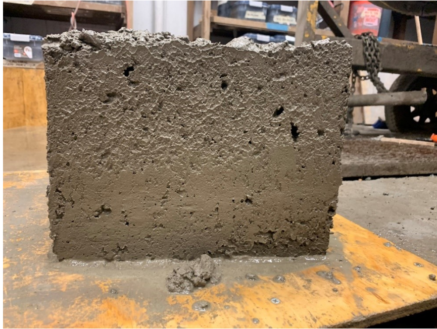
Figure A.16: Surface-void profile for one of the sides of box test specimen (Mixture 5)
