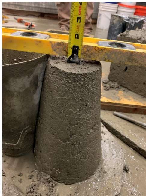
Figure A.31: Result from slump testing (Mixture 9)
