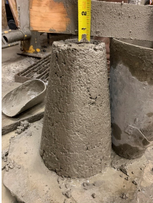
Figure A.14: Result from slump testing (Mixture 4)
