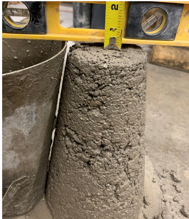
Figure A.42: Result from slump testing (Mixture 13)
