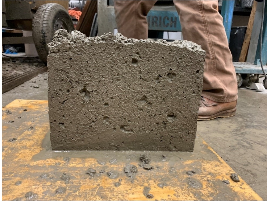
Figure A.12: Surface-void profile for one of the sides of box test specimen (Mixture 4)
