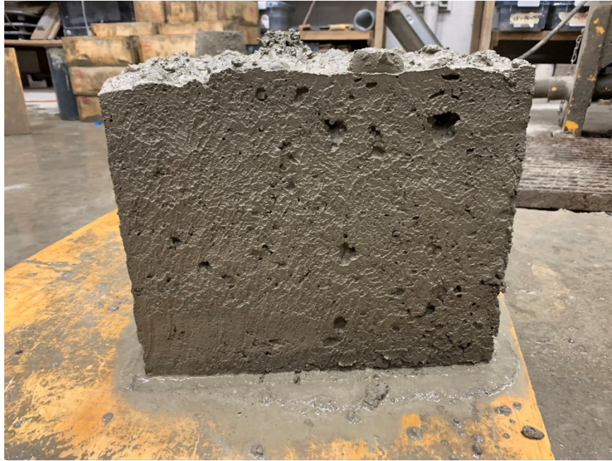
Figure A.33: Surface-void profile for one of the sides of box test specimen (Mixture 10)
