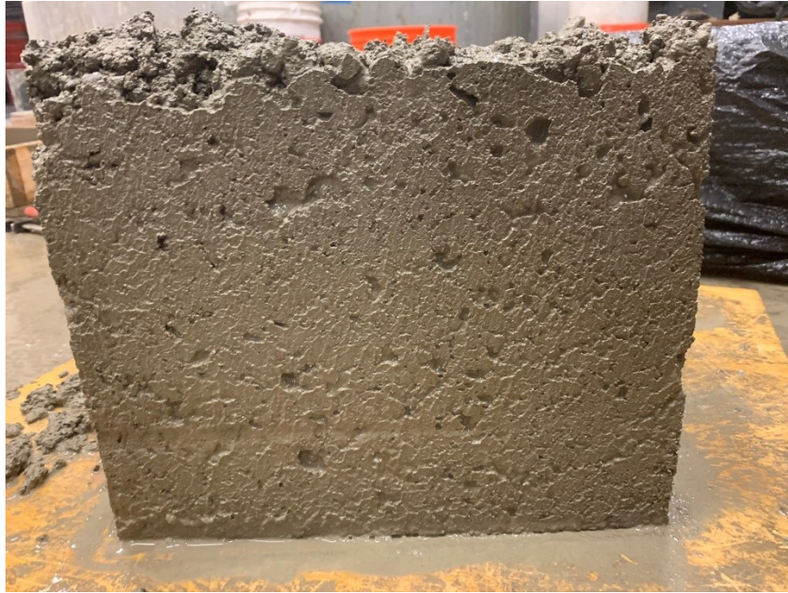
Figure A.44: Surface-void profile for one of the sides of box test specimen (Mixture 14)
