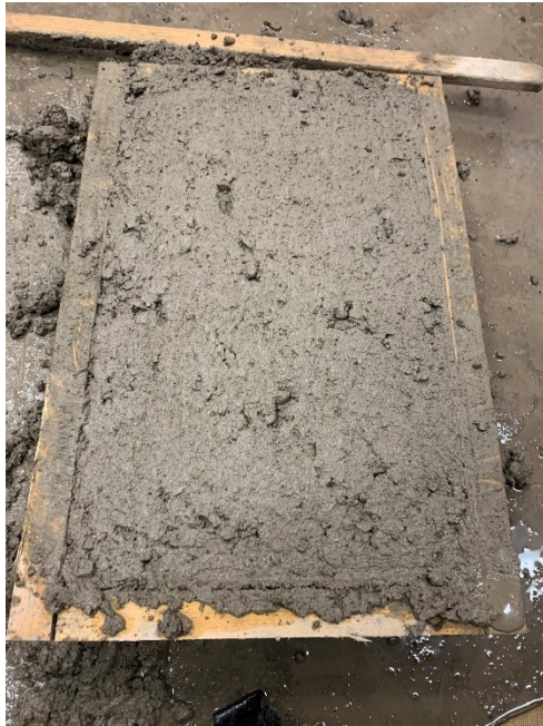
Figure A.23: Concrete finished surface after screeding and troweling (Mixture 6)
