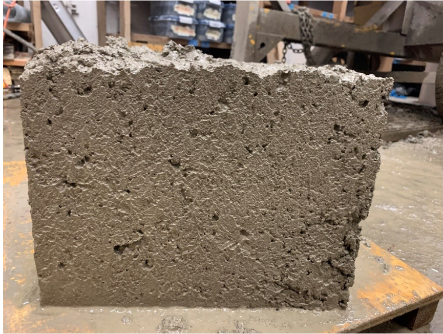
Figure A.24: Surface-void profile for one of the sides of box test specimen (Mixture 7)
