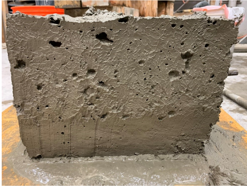
Figure A.52: Surface-void profile for one of the sides of box test specimen (Mixture 18)
