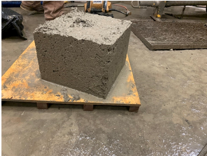
Figure A.21: Overview of box test specimen (Mixture 6)
