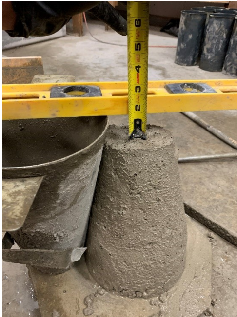
Figure A.40: Result from slump testing (Mixture 12)
