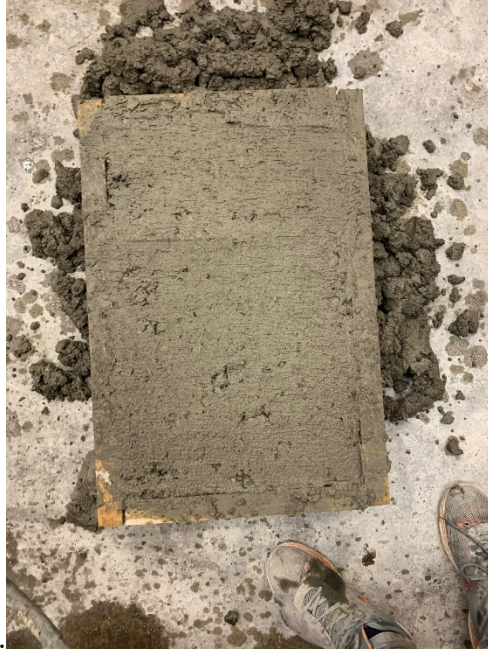
Figure A.54: Concrete finished surface after screeding and troweling (Mixture 18)
