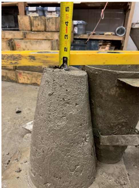
Figure A.34: Result from slump testing (Mixture 10)
