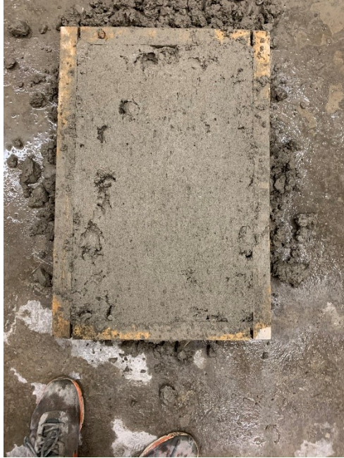
Figure A.35: Concrete finished surface after screeding and troweling (Mixture 10)
