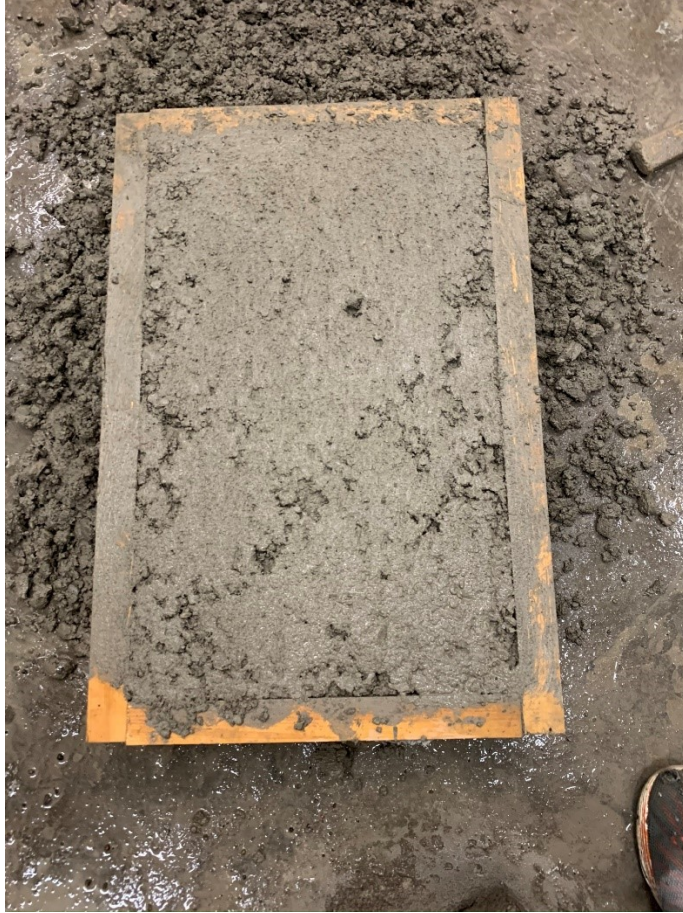
Figure A.43: Concrete finished surface after screeding and troweling (Mixture 13)
