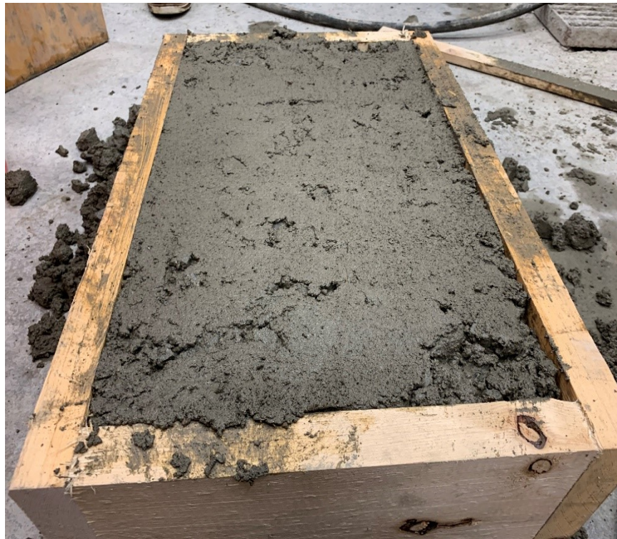
Figure A.4: Concrete finished- surface after screeding and troweling (Mixture 1)
