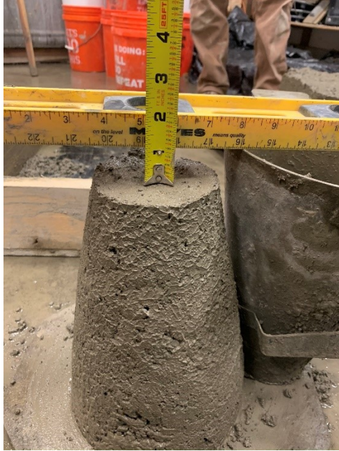
Figure A.22: Result from slump testing (Mixture 6)
