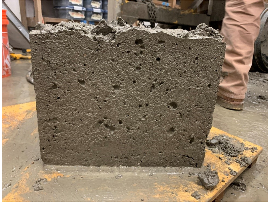
Figure A.30: Surface-void profile for one of the sides of box test specimen (Mixture 9)
