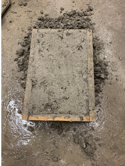
Figure A.32: Concrete finished surface after screeding and troweling (Mixture 9)
