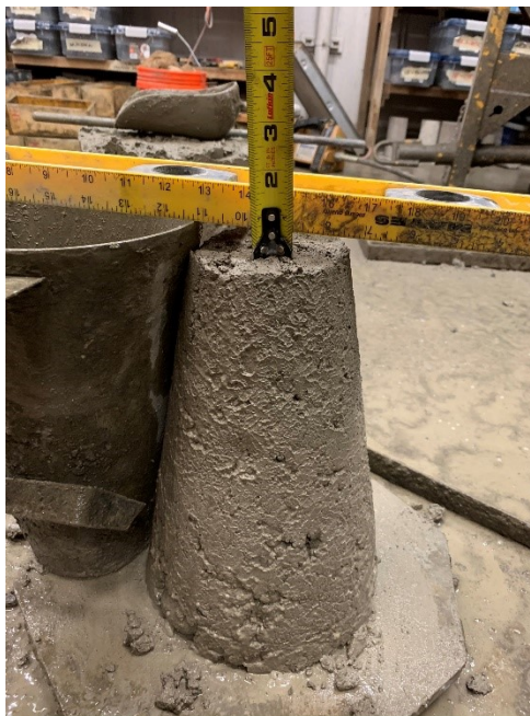
Figure A.37: Result from slump testing (Mixture 11)
