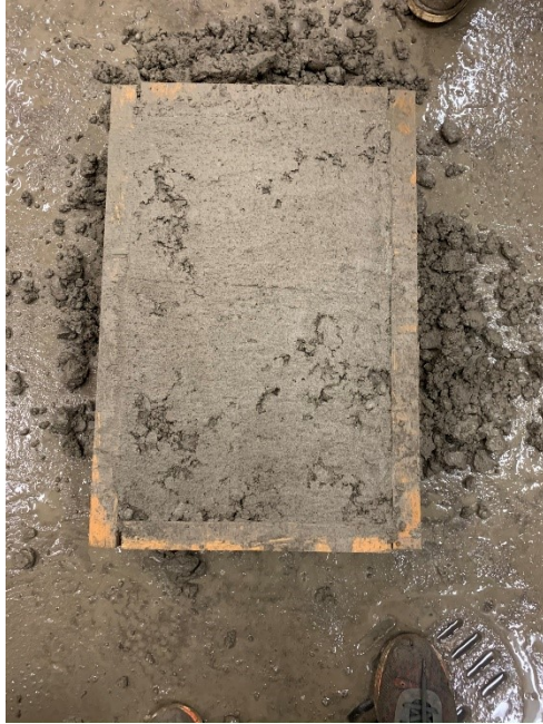
Figure A.51: Concrete finished surface after screeding and troweling (Mixture 17)
