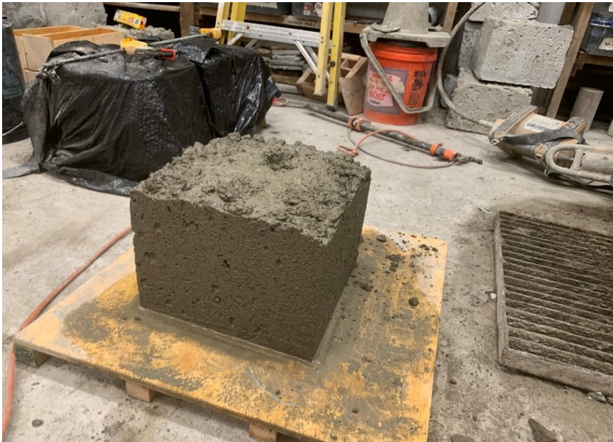
Figure A.2: Overview of box test specimen (Mixture 1)
