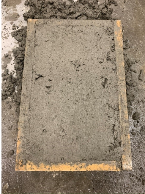
Figure A.29: Concrete finished surface after screeding and troweling (Mixture 8)
