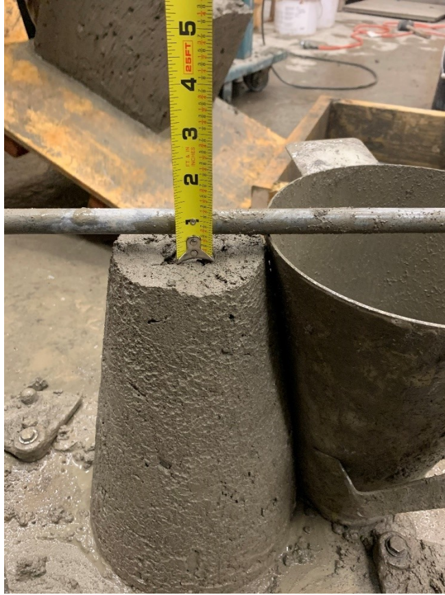
Figure A.10: Result from slump testing (Mixture 3)
