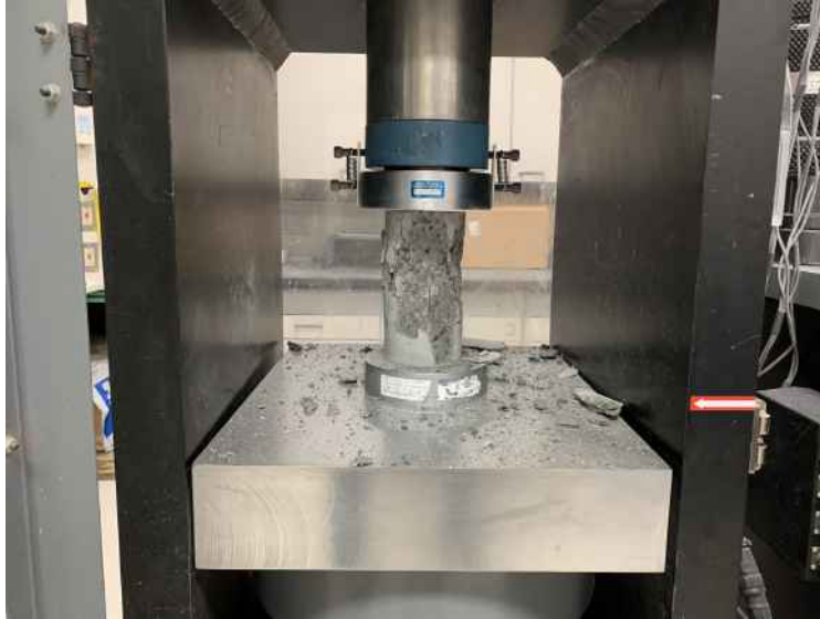
Figure 8 Failure of concrete cylinder in compression
