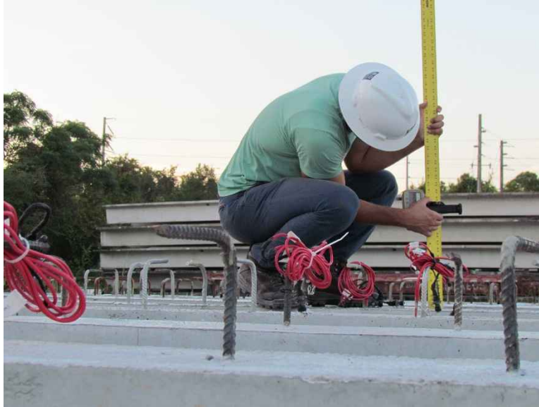
Figure 19 Adjusting the detector along the measuring ruler
