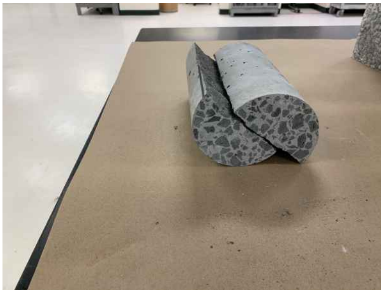
Figure 13 Tensile failure of cylinder
