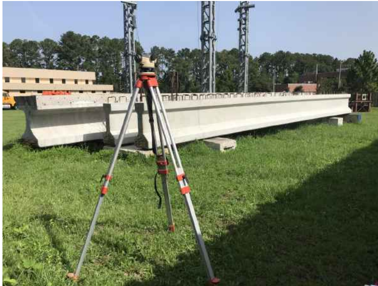
Figure 21 Measuring camber at the FDOT lab
