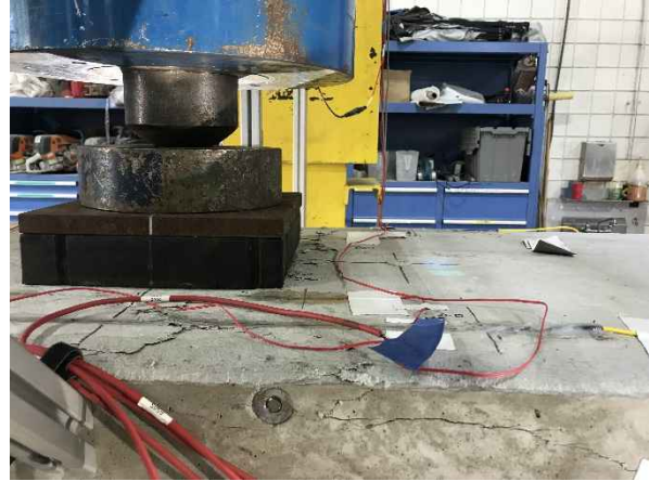
Figure 10-27 Crushing of concrete of Girder A3_1
