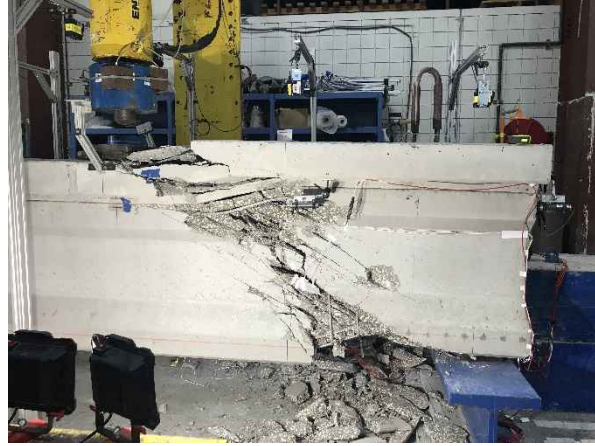
Figure 10-32 Web shear failure of Girder B3_2
