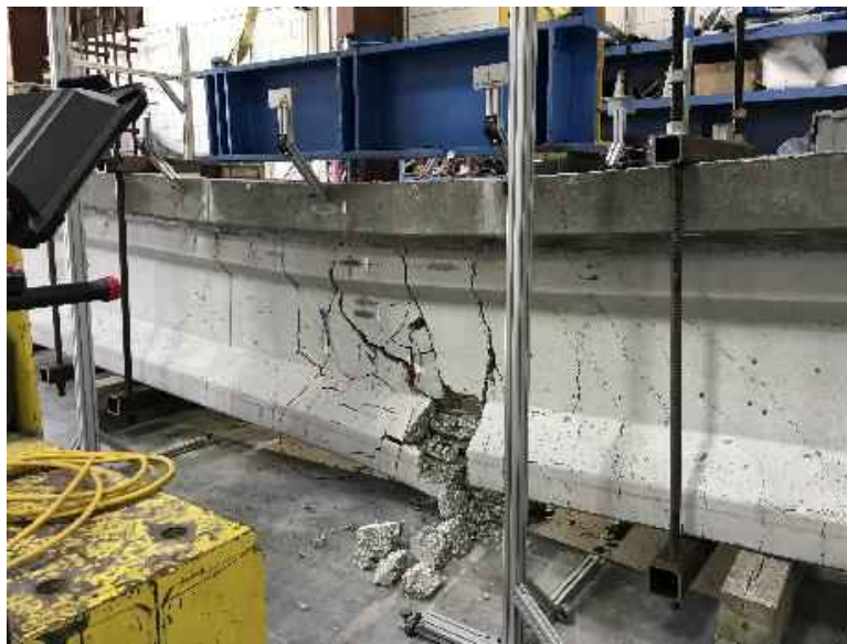
Figure 6-15 Rupture of strands failure mode (Girder B2)
