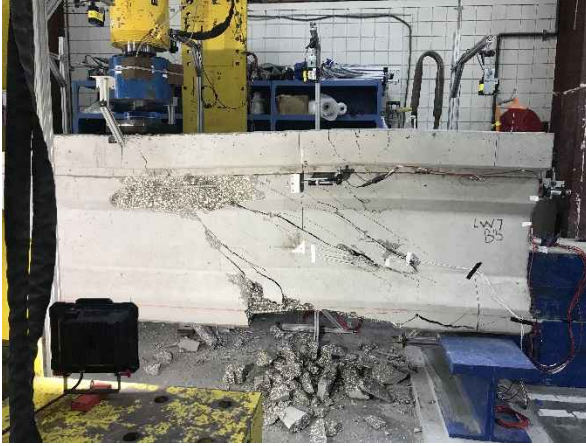
Figure 10-31 Web shear failure of Girder B3_1
