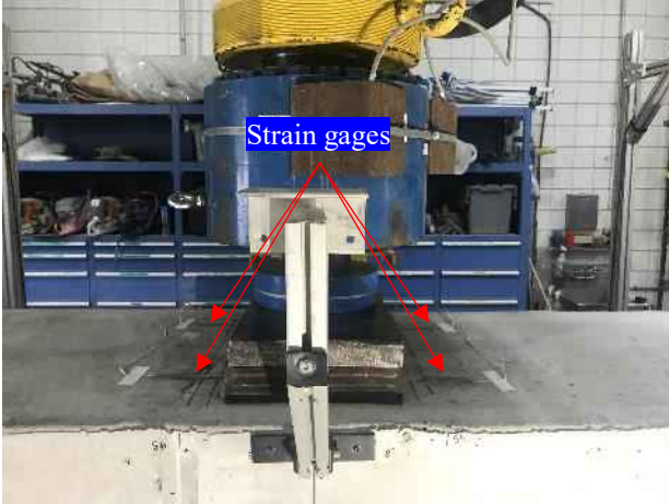
Figure 10-6 Strain gages at the top of the slab
