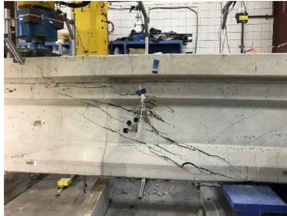
Figure 10-22 Girder A2_3 at failure
