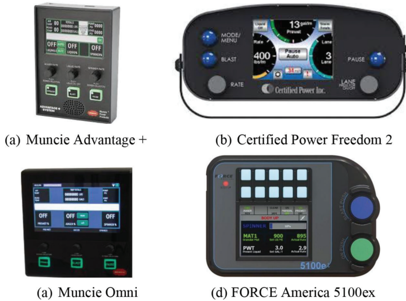
Figure 2.2 INDOT application controllers.
