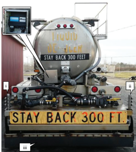
(b) Equipment Adaptation on 5,500-gallon Brine Tanker
