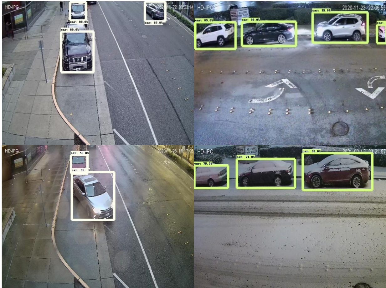
Figure 4-6 Sample Practical Test Result in City of Bellevue for Vehicle Detection in Different Conditions (Daylight, Night Vision, Rainy, and Snowy)
