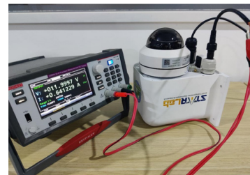
(c) Electric Surges Tests
