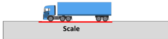
Figure 39a: Calibration Truck Weighing Procedure (GVW)
