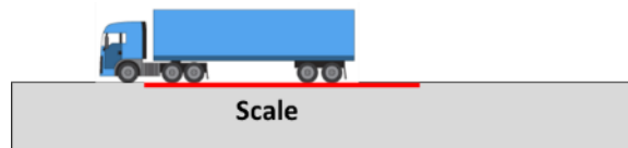
Figure 40a: Calibration Truck Weighing Procedure (Wb)
