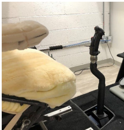
a) McFadden Series 292A 2-axis (pitch and roll) fighter stick
