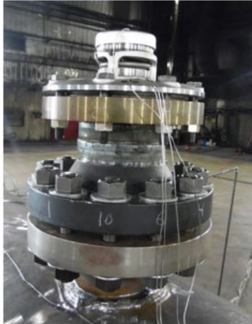
Test # 1 - Low capacity PRD mounted in upright orientation
