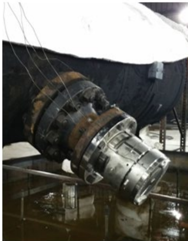
Test # 3 - High capacity PRD mounted at 120° orientation
