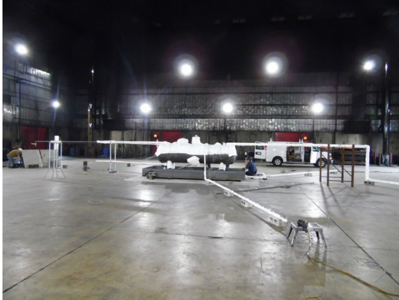
Figure 12. PRD fire test vessel with insulation
