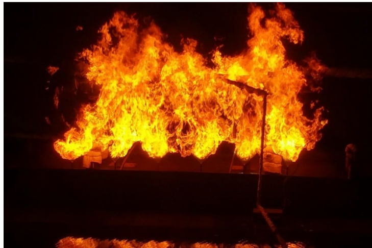
Figure 15. Vessel engulfed in fire-water tests
