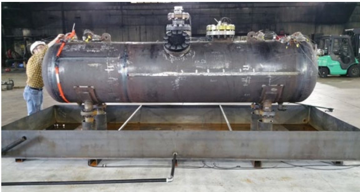
Figure 11. Test vessel sitting in fire pan, with PRD mounted on top, center nozzle
