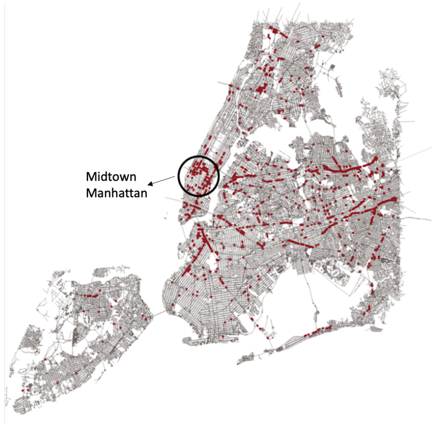
Figure 10. The top 1% congested links by v/c ratio at 8–9 a.m. in the base scenario.
