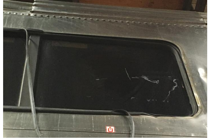
Figure 3. Zip-strip and gasket condition after Cimarron accident
