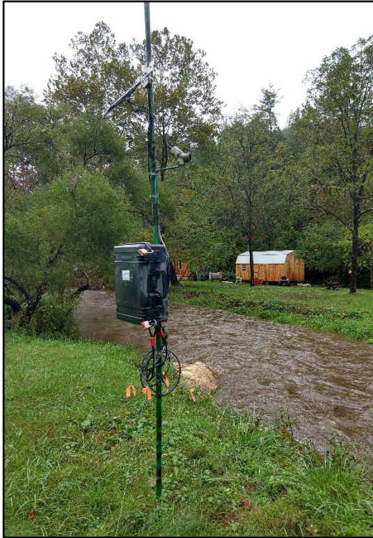
Figure 9. Examples of acoustic stations used to survey for foraging gray bats across the French Broad River Basin in western North Carolina. Big Laurel Station at left and Swannanoa River Station at right. Typically, two Anabat SD1 or SD2 units, housed with batteries in a water-tight case, were operational at each station. Microphones, mounted on the same or separate posts, were oriented such that one pointed upstream and the other pointed downstream.
