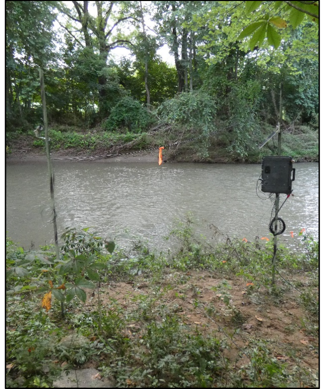
Figure 9. Examples of acoustic stations used to survey for foraging gray bats across the French Broad River Basin in western North Carolina. Big Laurel Station at left and Swannanoa River Station at right. Typically, two Anabat SD1 or SD2 units, housed with batteries in a water-tight case, were operational at each station. Microphones, mounted on the same or separate posts, were oriented such that one pointed upstream and the other pointed downstream.
