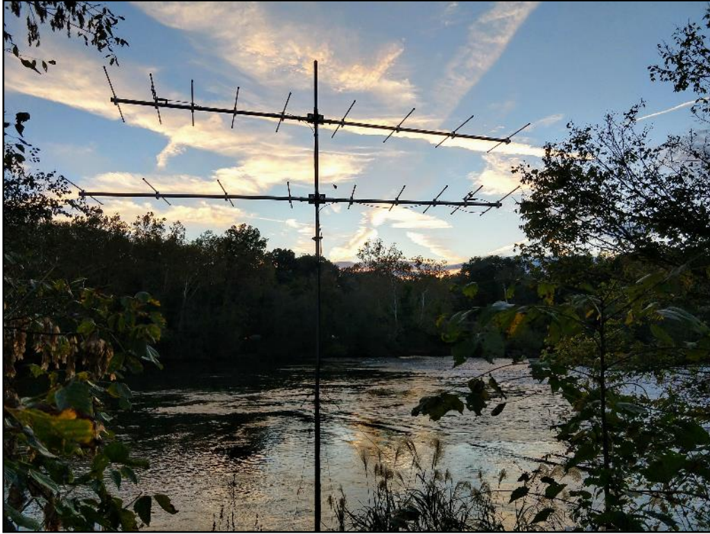
Figure 6. Fixed telemetry tower (N1) alongside the French Broad River in Asheville, North Carolina. One 9-element antenna points downstream and one points upstream. The antennae are connected to a datalogging receiver stored in a watertight case and powered by rechargeable batteries, sometimes in conjunction with a solar panel.
